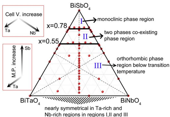
**Fig. 1.** Pseudo-phase diagram of  $\text{Bi}(\text{Sb}_x\text{Nb}_y\text{Ta}_z)\text{O}_4$  ( $x + y + z = 1$ ) system (I – monoclinic phase region below the melting point, III – orthorhombic phase region below transition temperature (in fact this region must be studied as a function of sintering temperature as discussed in paragraph “Results and discussions”), II – monoclinic and orthorhombic co-existing phase region below the melting point, M.P. – melting point, cell V – cell volume).
