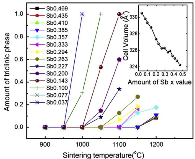
**Fig. 4.** Amount of triclinic phase in  $\text{Bi}[\text{Sb}_x(\text{Nb}_{0.5}\text{Ta}_{0.5})_{1-x}]\text{O}_4$  ( $0.037 \leq x \leq 0.469$ ) ceramics as a function of sintering temperature.
