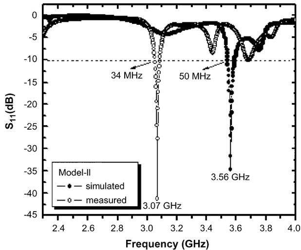
Fig. 3. The simulated and measured  $S_{11}$  parameters of model II.
