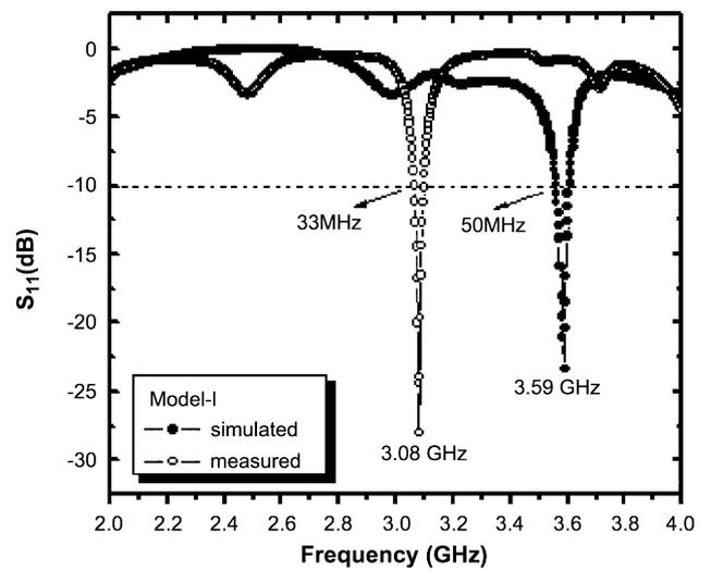
Fig. 2. The simulated and measured S<sub>11</sub> parameters of the model I.
