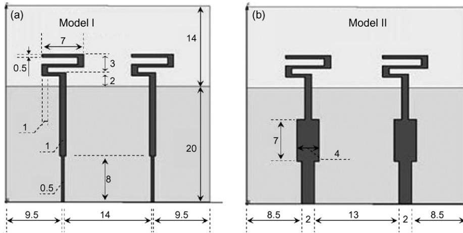
Fig. 1. The geometry of the two-element array printed on the BiNbO<sub>4</sub> ceramic substrate.
