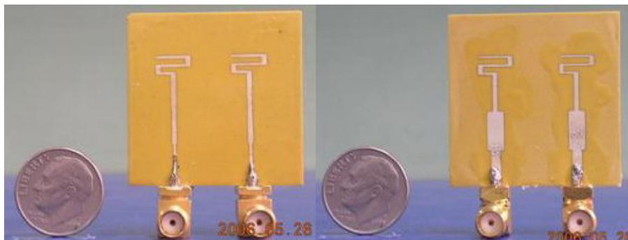
Fig. 5. Real photos of antenna samples based on  $\text{BiNbO}_4$  ceramic substrate.
