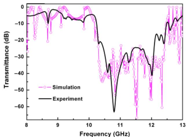
Fig. 4. The measurement (solid line) and simulation results (dash dotted line) of the combined photonic crystal with the period change 134%.
