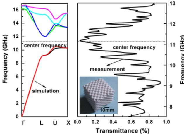
Fig. 1. The simulation and measurement results of the perfect three-dimensional photonic crystals with dimension of 60 mm × 60 mm × 60 mm.
