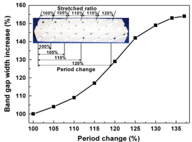
Fig. 3. The measurement result of the relationship between the band gap width and the period change of the combined photonic crystal (PC) with uniting the separate stretched PCs.
