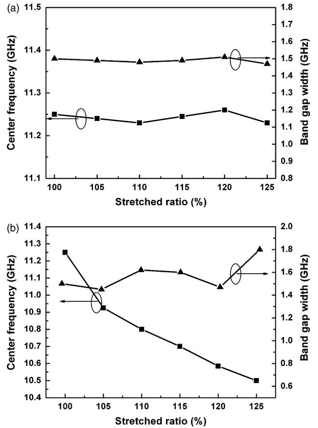
Fig. 2. The band gap properties relative with the stretching of the photonic crystals in vertical (a) and parallel (b) to the propagation of the electromagnetic wave.
