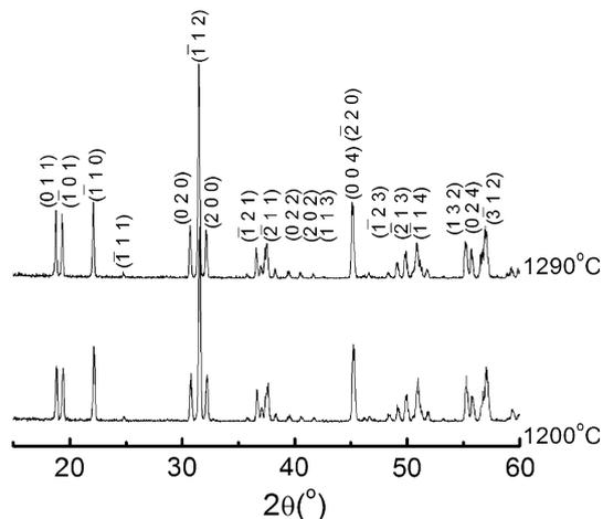
**Fig. 1** XRD patterns of  $\text{Ca}_3\text{WO}_6$  ceramics sintered at 1,200 and 1,290 °C for 2 h
