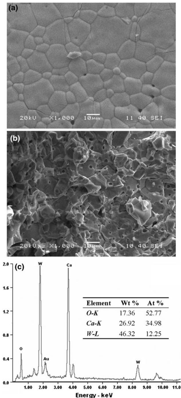
**Fig. 3** SEM micrographs of as-fired surface **a**, fractured surface **b** and EDS spectrum **c** of  $\text{Ca}_3\text{WO}_6$  ceramics sintered at 1,275 °C for 2 h
