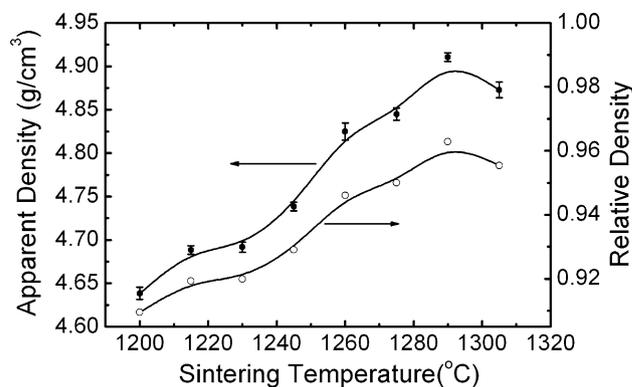
**Fig. 2** Apparent density and relative density of  $\text{Ca}_3\text{WO}_6$  ceramics sintered at different temperatures
