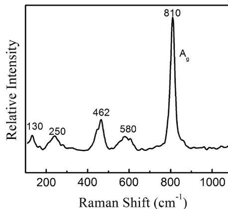
**Fig. 4** Raman spectrum of  $\text{Ca}_3\text{WO}_6$  ceramic sintered at 1,275 °C for 2 h
