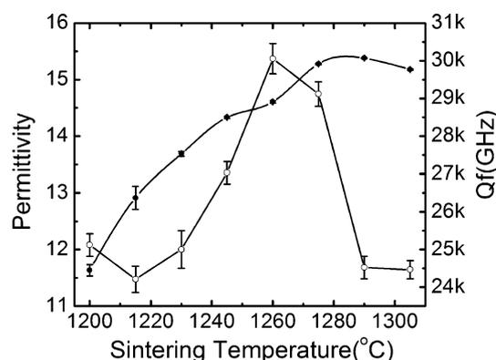
**Fig. 5** Microwave dielectric constant and Qf values of  $\text{Ca}_3\text{WO}_6$  ceramic as a function of sintering temperature
