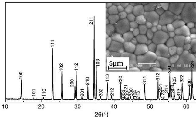
Fig. 1. XRD pattern and SEM micrograph (the insert part) of  $\text{LiZnNbO}_4$  ceramic sintered at 950 °C.
