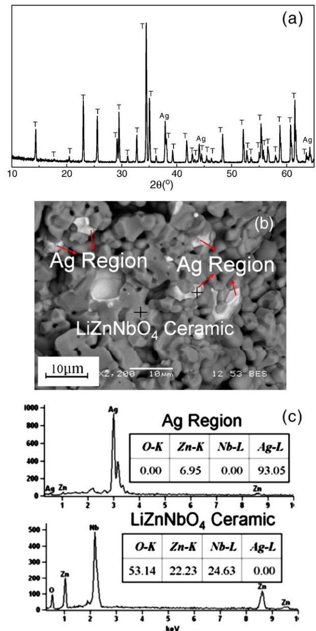
Fig. 2. XRD pattern (a), BEI micrograph (b) and EDS spectrums (c) of the fractured surface of the co-fired ceramic ( $\text{LiZnNbO}_4$  with 20 wt.% Ag powders sintered at 950 °C for 3 h).
