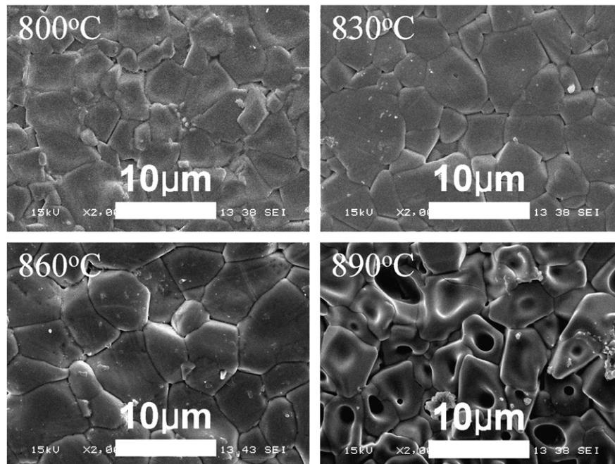
**Fig. 2.** SEM photos of  $\text{BaLa}_2(\text{MoO}_4)_4$  ceramics sintered at 800–890 °C for 2 h.
