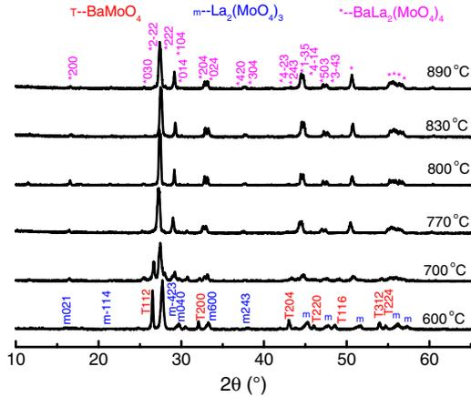
**Fig. 1.** XRD patterns of the  $\text{BaLa}_2(\text{MoO}_4)_4$  ceramics calcined and sintered at different temperatures.
