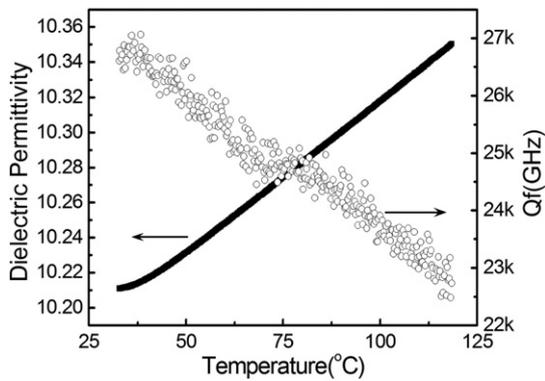
Fig. 3. Microwave dielectric permittivity and Qf values of  $\text{BaLa}_2(\text{MoO}_4)_4$  ceramic vs temperature.
