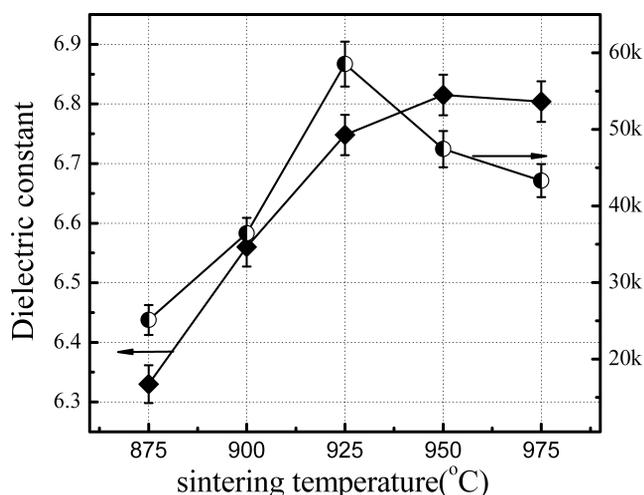
Fig. 3. The dielectric constant and  $Q \times f$  values of Zn<sub>3</sub>B<sub>2</sub>O<sub>6</sub> ceramics as a function of sintering temperature.
