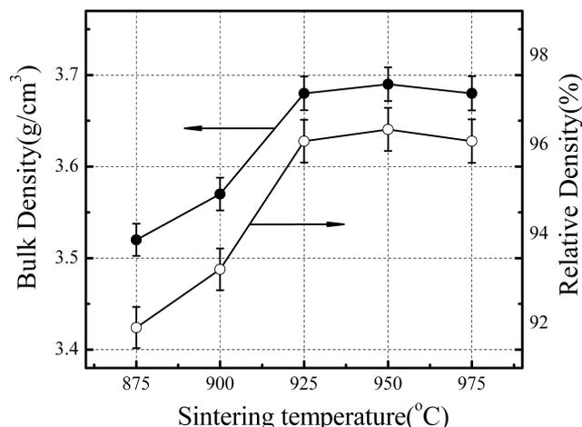
Fig. 2. Bulk densities of Zn<sub>3</sub>B<sub>2</sub>O<sub>6</sub> ceramics as a function of sintering temperatures.
