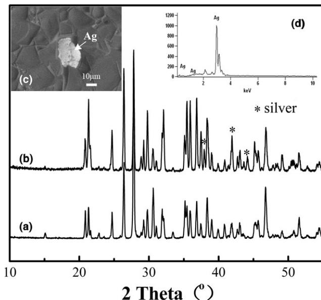
**Fig. 4.** The XRD result of the  $\text{Zn}_3\text{B}_2\text{O}_6$  ceramic sintered at  $925^\circ\text{C}$  for 4 h (a) and XRD results (b), Backscattered electron imaging micrographs (c) and EDS analysis (d) of the  $\text{Zn}_3\text{B}_2\text{O}_6$  ceramic co-fired with 20 wt% silver (Ag) addition at  $950^\circ\text{C}$  for 2 h.
