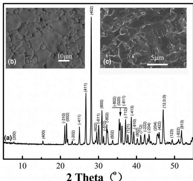
Fig. 1. The XRD result (a), SEM of the surface (b), cross section (c) of Zn<sub>3</sub>B<sub>2</sub>O<sub>6</sub> ceramic sintered at 925°C for 4 h.
