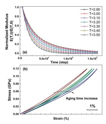
FIG. 10. (Color online) (a) Calculated elastic modulus and (b) stress-strain curves as a function of deaging time in the parent phase. The decrease of the elastic modulus and the flattening of the stress-strain curves in the parent phase with deaging time are the predictions from our calculation. The elastic moduli are normalized by the initial values through E(T,t)/E(T,0).
