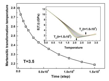
FIG. 8. (Color online) Parent phase stabilization effect: decrease of the martensitic transformation temperature with deaging time at temperature T=3.5. The inset contains the elastic modulus vs temperature curves for different deaging times for T=3.5 showing that the dip temperature of the elastic modulus shifts to the low-temperature side with deaging in the parent phase.
