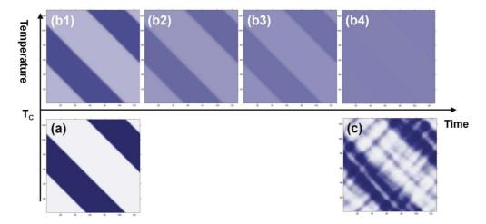
FIG. 9. (Color online) Domain evolution during a heating and cooling cycle and deaging with time in the parent phase. A typical domain pattern of aged martensite (a) was heated up to the parent phase (b1) where residual domain contrast remains. With deaging in the parent phase, such domain contrast gradually disappears [(b1)–(b4)]. After quenching to martensite again, a new domain pattern (c) is observed.
