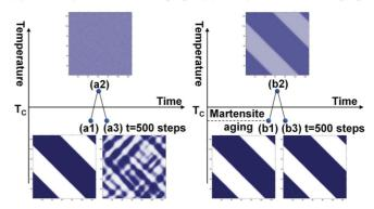
FIG. 5. (Color online) The domain evolution during temperature-induced martensitic transformation. For unaged martensite, a typical domain pattern (a1) was heated to the parent phase (a2), followed by a quench to martensite (a3). The domain pattern cannot be memorized. For aged martensite, a typical domain pattern (b1) was heated to the parent phase (b2) followed by a quench to martensite (b3). The same domain pattern as (b1) is restored.
