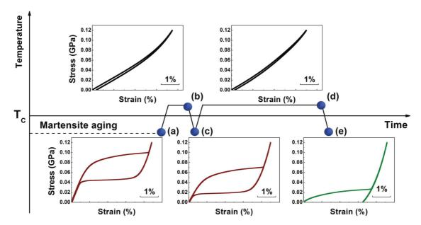
FIG. 7. (Color online) Evolution of the deformation behavior during a heating and cooling cycle for aged martensite. (a) Pseudoelastic, rubberlike behavior of the aged martensite. The sample was heated up to (b) the parent phase and cooled down to (c) the martensite phase with RLB. The sample was then heated up again to (d) the parent phase and held for  $1.0 \times 10^6$  simulation steps, followed by cooling down to (e) where the refreshed martensite exhibits normal plastic behavior.
