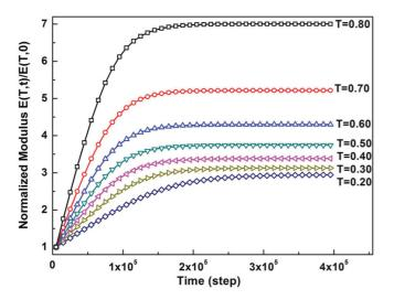
FIG. 6. (Color online) Elastic modulus as a function of aging time at different temperatures showing that an increase of temperature stiffens the system, and aging at a given temperature leads to rubberlike behavior. The elastic moduli are normalized by the initial values through E(T,t)/E(T,0).
