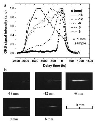
**Fig. 2.** (a) Time-resolved two-color OKS signals, and (b) recorded images of the formed filament in the sample, when the 10-mm-thick sample was fixed at different positions. The pump power was fixed at 3 mW.
