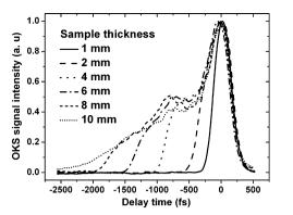
Fig. 3. Time-resolved two-color OKS signals for glasses with different thicknesses.
