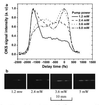
**Fig. 4.** (a) Time-resolved two-color OKS signals for different pump powers, and (b) recorded images of the formed filament in the 10-mm-thick glass.
