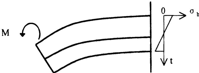
FIGURE 3 Schematic diagram of imagined couple M and thermal bending stress \sigma_b
