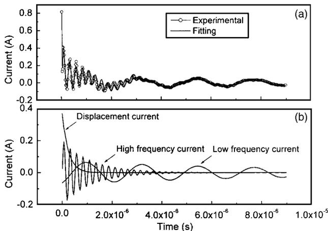
FIG. 5. Experimental and fitting data of modified PZT ceramic. ( $E = 6 \text{ kV/cm}$ ) (a) total current of the fitting and experimental data, (b) three branches of total current.
