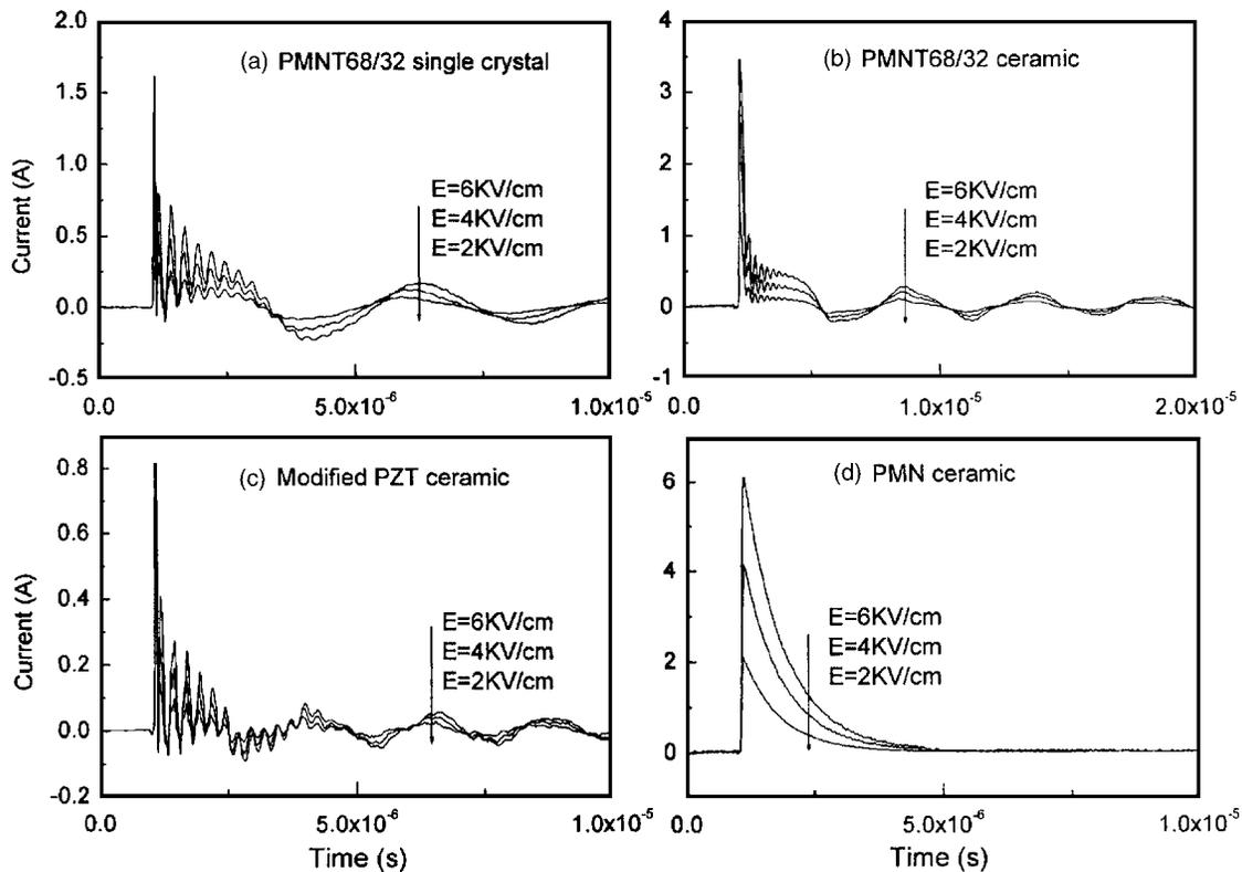
FIG. 2. Transient currents as a function of time for various ferroelectrics. (a) PMNT 68/32 single crystal, (b) PMNT 68/32 ceramic, (c) modified PZT ceramic, (d) PMN ceramic.
