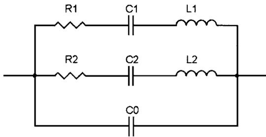
FIG. 4. Equivalent electrical circuit of a ferroelectric specimen.
