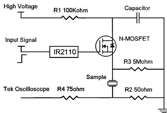
FIG. 1. Schematic circuit diagram of test platform. The current is measured across a series resistor, using an oscilloscope operated in the time capture mode.
