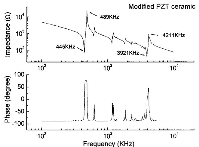
FIG. 3. Impedance of modified PZT ceramic as a function of frequency.
