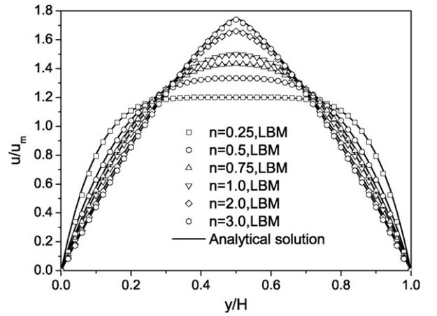
Fig. 1. Comparisons between the LBM results and the analytical solutions in the pressure-driven non-Newtonian flow.
