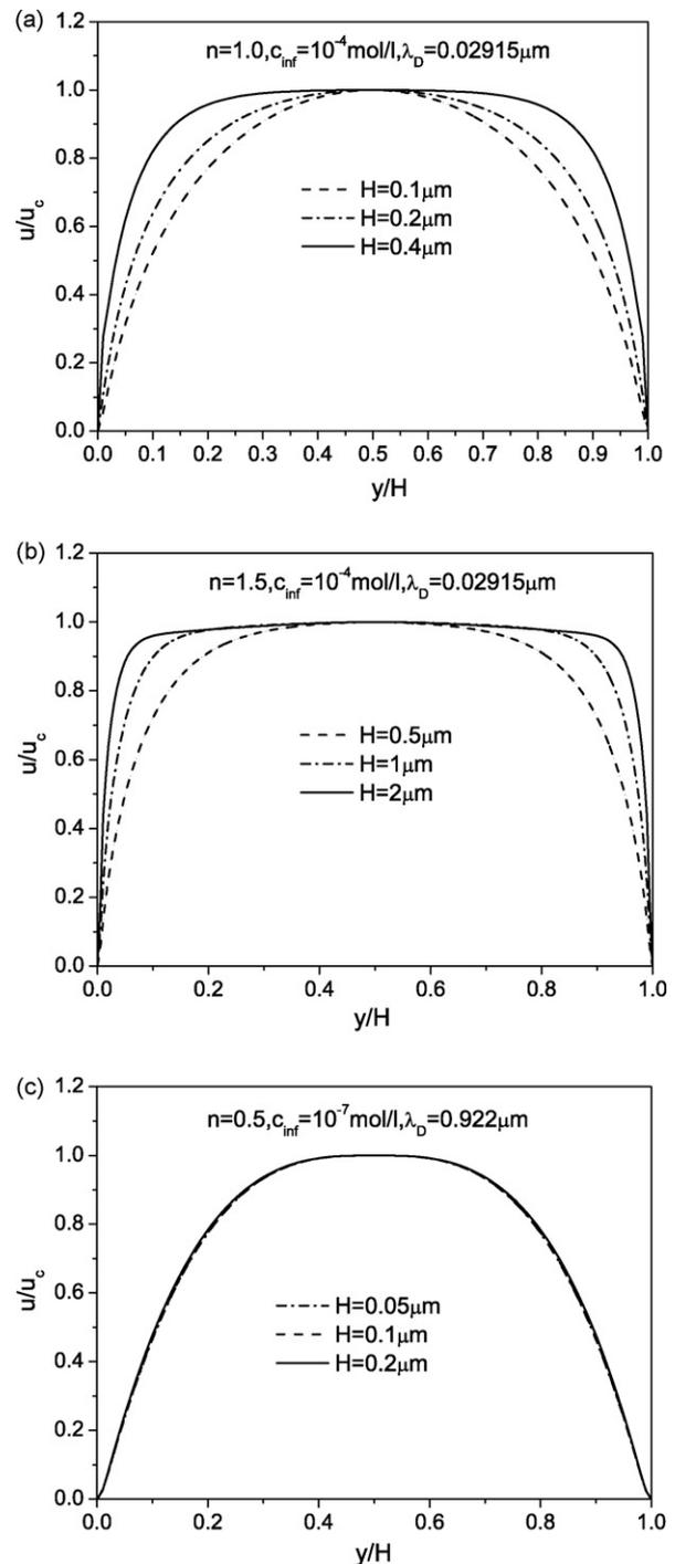
**Fig. 3.** Normalized velocity profiles for various channel heights at different ionic concentrations and power-law exponents  $n$  in the electroosmotic flow. (a)  $n = 1.0$ ,  $c_{inf} = 10^{-4}$  mol/l. (b)  $n = 1.5$ ,  $c_{inf} = 10^{-4}$  mol/l. (c)  $n = 0.5$ ,  $c_{inf} = 10^{-7}$  mol/l.
