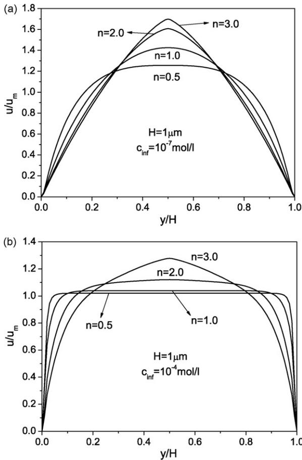
**Fig. 2.** Normalized velocity profiles for various power-law exponents  $n$  at two different ionic concentrations in the electroosmotic flow. (a)  $c_{inf} = 10^{-7}$  mol/l and (b)  $c_{inf} = 10^{-4}$  mol/l.
