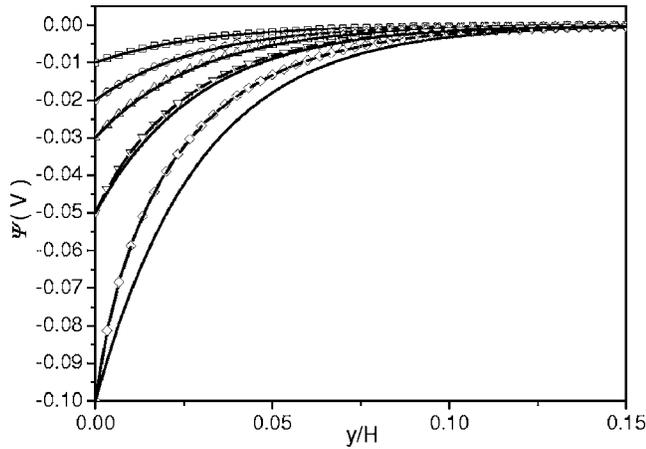
FIG. 2. The electric potential comparisons of the LBM results (open symbols), the solutions of the linearized Poisson-Boltzmann equation (solid lines), and the numerical results of the nonlinear Poisson-Boltzmann equation with the finite volume method (dashed lines).
