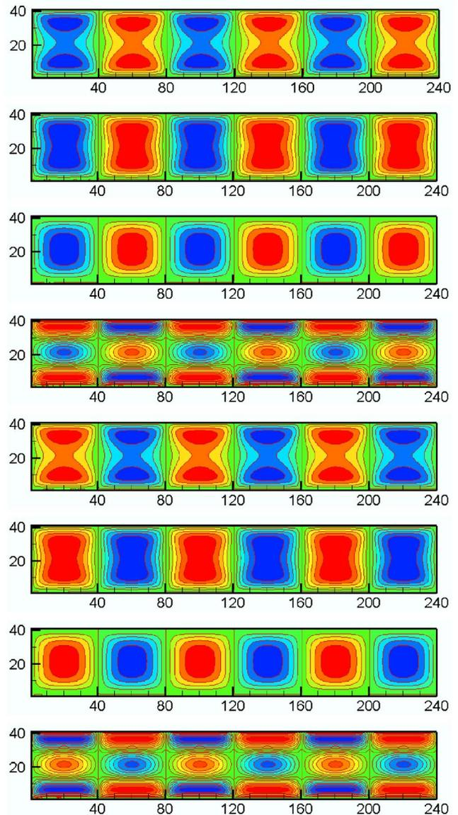
FIG. 10. (Color online) Streamlines at eight different times. From the upper to the bottom,  $t=0$ ,  $T_E/8$ ,  $T_E/4$ ,  $3T_E/8$ ,  $T_E/2$ ,  $5T_E/8$ ,  $3T_E/4$ , and  $7T_E/8$ .
