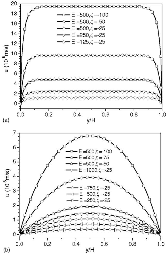
FIG. 4. The streamwise velocity profiles at various external electric field intensities and zeta potentials. (a)  $c_\infty = 10^{-4}$  mol/l. (b)  $c_\infty = 10^{-7}$  mol/l.
