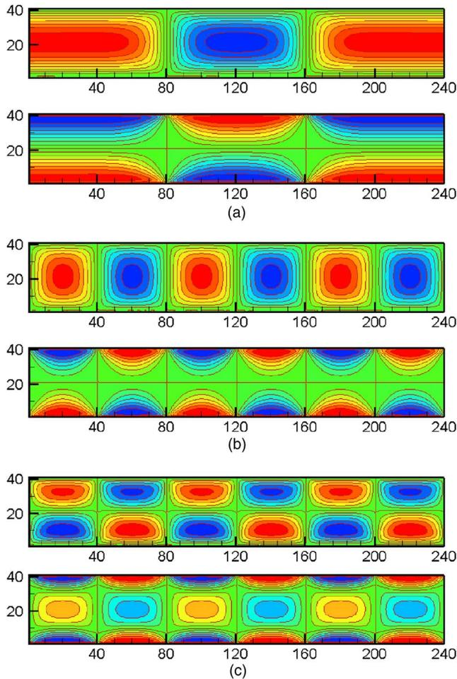
FIG. 9. (Color online) Streamlines (the upper) and isolines of the streamwise velocity (the bottom) for heterogeneous surface potential cases. (a) Case 1. (b) Case 2. (c) Case 3.
