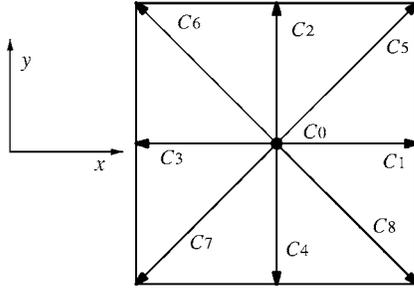
FIG. 1. Schematic of D2Q9 lattice.
