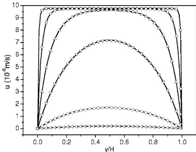
FIG. 5. The streamwise velocity profiles at various bulk ionic molar concentrations. From the bottom to the upper, the bulk ionic molar concentration is  $c_\infty = 10^{-8}, 10^{-7}, 10^{-6}, 10^{-5}, 10^{-4},$  and  $10^{-3}$  mol/l, respectively.
