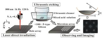
Fig. 1. Schematic diagram of microlens fabrication.
