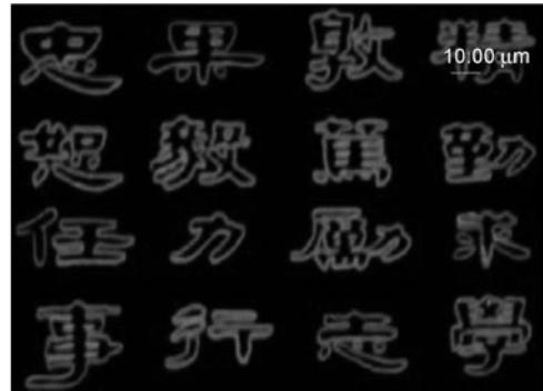
**Figure 5** The pattern of Xi'an Jiaotong University motto fabricated on a copper thin film.
