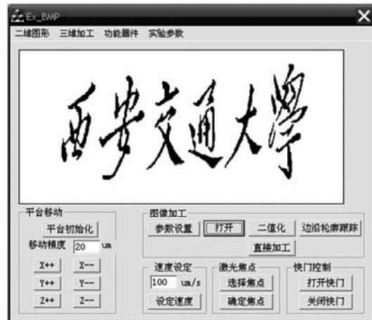
Figure 2 The control interface of femtosecond laser micromachining software.
