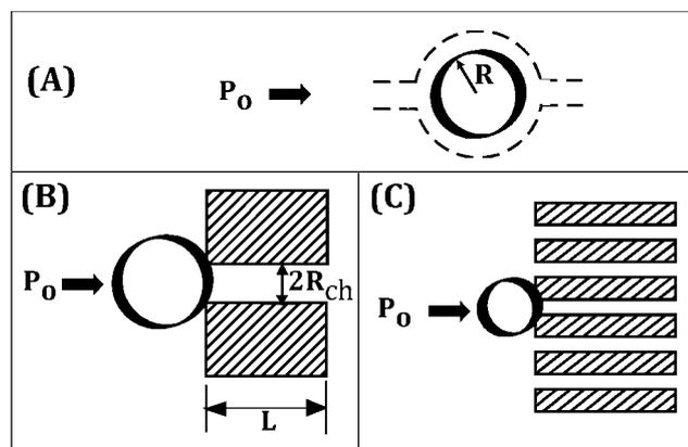
**Fig. 2** Various flow configurations that can affect cell pressure: (A) shear flow past a spherical cell; (B) a cell completely occludes an aperture (0-D); (C) a cell completely occludes an aperture in the presence of other unobstructed apertures (0-D).
