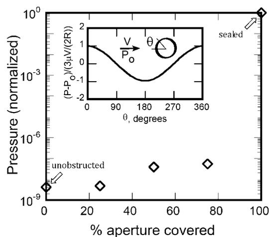
**Fig. 3** Cell pressure as a function of the percent area of an aperture blocked. Data points were obtained by solving the Navier–Stokes equation numerically for a 5  $\mu\text{m}$  (D)  $\times$  10  $\mu\text{m}$  (L) channel partially blocked by a 5  $\mu\text{m}$  (D) cell, at a fluid velocity of 1  $\mu\text{m s}^{-1}$ . **Inset:** Pressure distribution from a flow around a spherical object. Zero degree is defined as the angle opposite of the upstream flow direction.
