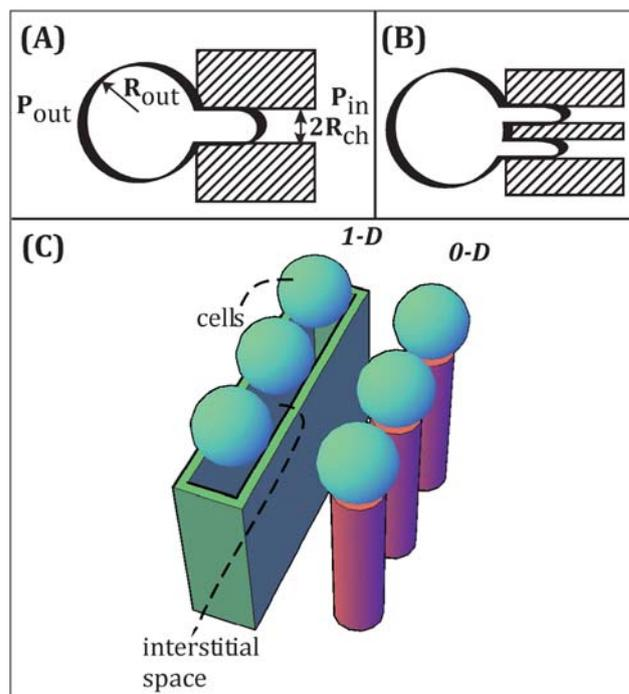
**Fig. 4** (A) A channel of diameter  $2R_{ch}$  completely clogged by a cell with the external radius  $R_{out}$ . (B) Two channels simultaneously clogged by a cell. (C) 1-D aperture versus 0-D aperture under high-density cell blockage. 1-D apertures offer interstitial spaces for bypass flow even in close-packing configuration whereas 0-D apertures do not.
