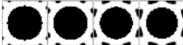
Fig.6 Topology of the bi-material plate (white: material 0; black: material 1) of the case f=250\text{Hz} in the four thermal environments a \Delta T = 0^\circ\text{C} , b \Delta T = 50^\circ\text{C} , c \Delta T = 75^\circ\text{C} , d \Delta T = 90^\circ\text{C} (from left)
