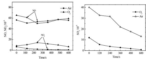
Fig4. Comparison of NO<sub>x</sub> & SO<sub>2</sub> emission value with different gasification medium
