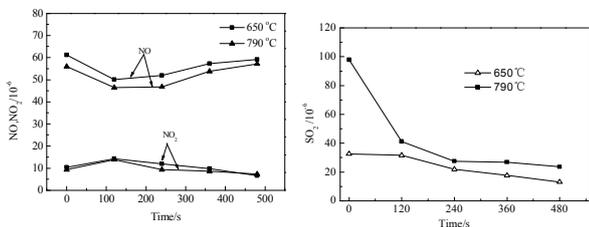
Fig3. Comparison of NO<sub>x</sub> & SO<sub>2</sub> emission values with different temperature
