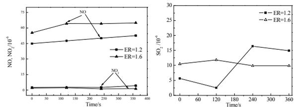
Fig6. Comparison of NO<sub>x</sub> & SO<sub>2</sub> emission under different work conditions
