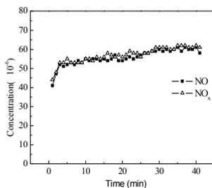
Fig2. Curves of NO<sub>x</sub> emission from combustion without sample in gasifier
