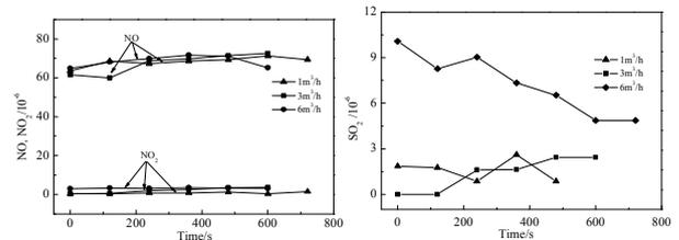
Fig5. Comparison of NO<sub>x</sub> & SO<sub>2</sub> emission value with different gas flow rate
