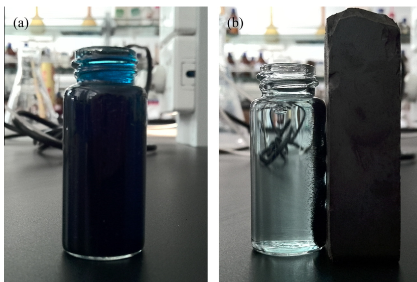
Fig. 8. Photos of recyclability tested by a magnet: (a) before adsorption and (b) separation using a magnet after adsorption.
