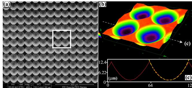
Fig. 3. Morphological observation of MLA with a fill factor of 78.0%. (a) SEM image of uniform MLA. (b) 3D-confocal analysis of marked region in (a). (c) Cross-sectional profile analysis of marked position in (b); y axis (etch depth) was stretched relative to x axis to show the profile more clearly.
