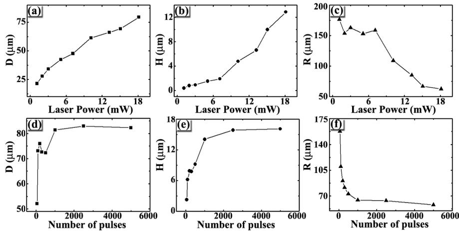
Fig. 4. Dependences of  $D$ ,  $H$ , and  $R$  values of microlenses on (a), (b), and (c) femtosecond laser power and (d), (e), and (f) number of pulses. Etching time was 40 min.  $D$ ,  $H$ , and  $R$  were measured by confocal microscopy.
