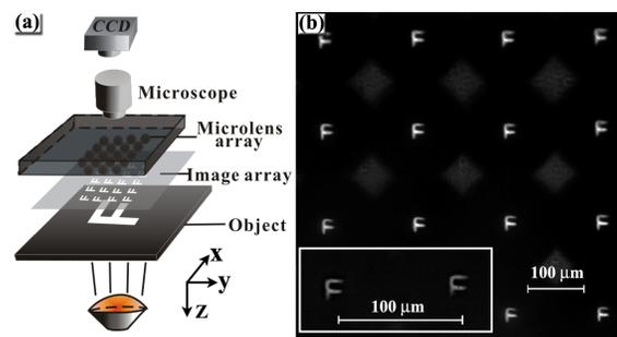
Fig. 5. Process of imaging MLA with a fill factor of 96.6%. (a) Imaging device. (b) Image array made by the MLA.
