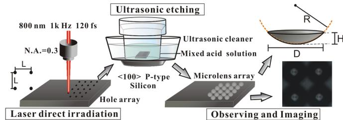
Fig. 1. Schematic diagram of microlens fabrication.
