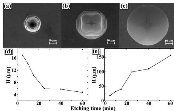
Fig. 2. SEM images of microlenses with laser power of 7 mW and pulse number of 50 at etching times of (a) 1 min, (b) 5 min, and (c) 10 min. (d) Heights and (e) radii of curvature at successive times during etching.
