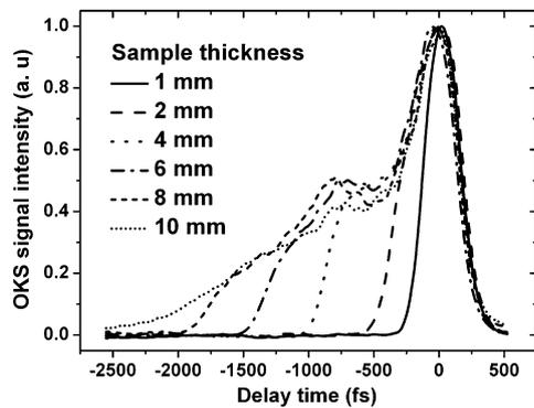
Fig. 3. Time-resolved two-color OKS signals for glasses with different thicknesses.
