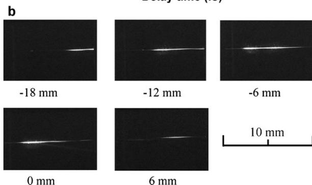
**Fig. 2.** (a) Time-resolved two-color OKS signals, and (b) recorded images of the formed filament in the sample, when the 10-mm-thick sample was fixed at different positions. The pump power was fixed at 3 mW.
