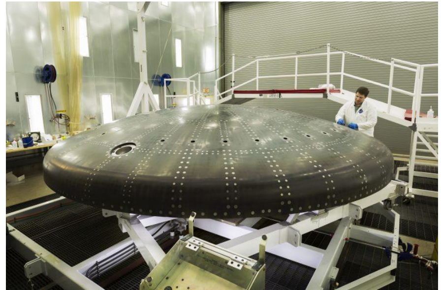
Heat shield composite structure for NASA's Orion spacecraft, over 4500° F re-entry temperatures, 16.5 feet in diameter
