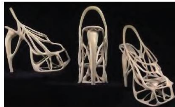
Melonia Shoe made by laser sintering, courtesy of Naim Josefi and Souzan Youssouf
