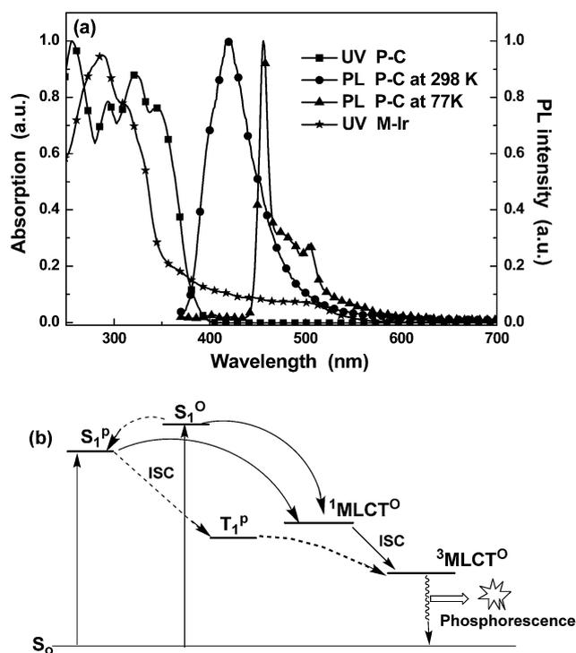
Fig. 2 (a) UV-Vis spectra for **P-C** and **M-Ir** together with the PL spectrum of **P-C** in  $CH_2Cl_2$  at both 298 K and 77 K. (b) Energy-transfer sketch involved in the orange phosphorescent polymers.
