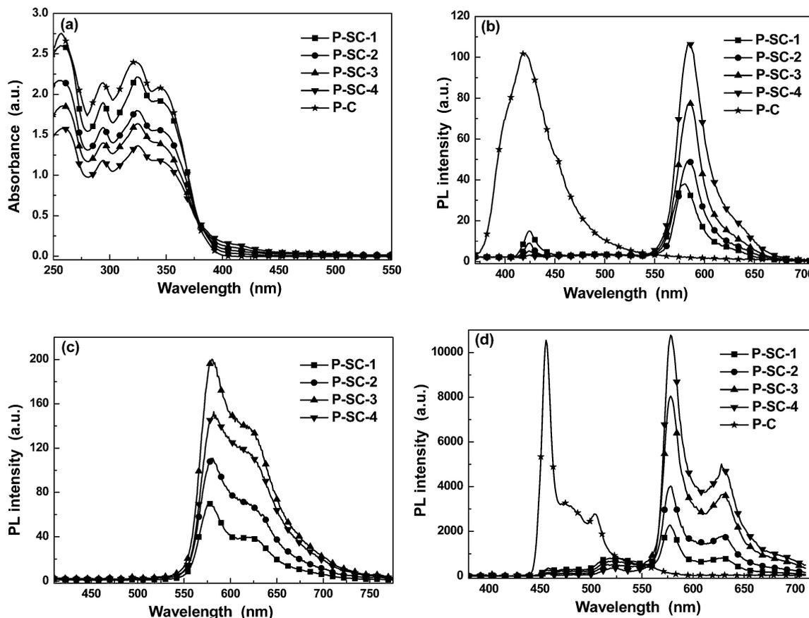
Fig. 1 (a) UV-Vis absorption spectra for the copolymers in  $\text{CH}_2\text{Cl}_2$  at 298 K. (b) The photoluminescent (PL) spectra for the copolymers in  $\text{CH}_2\text{Cl}_2$  at 298 K. (c) The PL spectra for the copolymer films at 298 K. (d) The PL spectra at 77 K for the copolymers in  $\text{CH}_2\text{Cl}_2$ .
