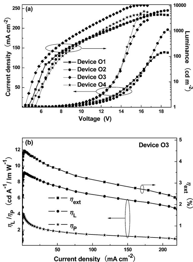
Fig. 5 (a) The current-density–voltage–luminance ( $J$ – $V$ – $L$ ) curves for all the devices. (b) The relationship between EL efficiencies and current density for device O3.
