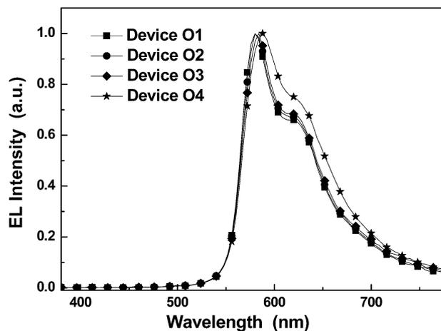
Fig. 4 The EL spectra for the solution-processed PHOLEDs at *ca.* 12 V.
