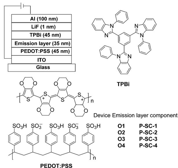
Fig. 3 The configuration of the PHOLEDs made from the orange phosphorescent polymers and the chemical structures for the involved functional materials.
