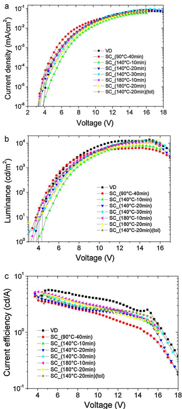
**Fig. 5.** Characteristics of solution processed and vacuum-deposited devices of ITO/PEDOT:PSS/TBADN+NPB:DPAVBi/BAIQ/Alq3/LiF/Al, respectively. (a) Current–density voltage, (b) luminance–voltage, and (c) current efficiency–voltage.
