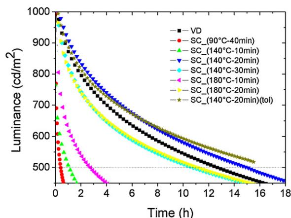
**Fig. 6.** Luminance decay versus time characteristics of solution processed (chlorobenzene and toluene (tol)) and vacuum-deposited devices of ITO/PEDOT:PSS/TBADN+NPB:DPAVBi/BAIQ/Alq3/LiF/Al structure (at an initial brightness of  $1000 \text{ cd/m}^2$ ).
