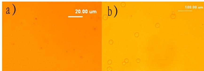
**Fig. 1.** The optical microscope images of organic films spin-coated on top of ITO. (a) All the images of the film annealed on the following conditions (90 °C, 40 min), (140 °C, 10 min), (140 °C, 20 min), (140 °C, 30 min), (180 °C, 10 min), (180 °C, 20 min) like the same, So one image was given to represent them; (b) annealing condition (220 °C, 10 min).
