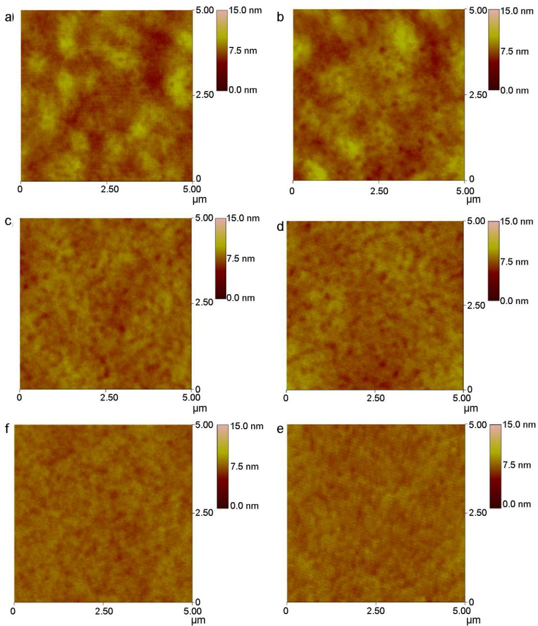
**Fig. 2.** The AFM images of spin-coated films with annealing condition of (a) 90 °C, 40 min (RMS=0.883 nm), (b) 140 °C, 10 min (RMS=0.870 nm), (c) 140 °C, 20 min (RMS=0.574 nm), (d) 140 °C, 30 min (Ra=0.596 nm), (e) 180 °C, 10 min (Ra=0.412 nm), and (f) 140 °C, 20 min (Ra=0.406 nm) (scan size: 5 μm × 5 μm).
