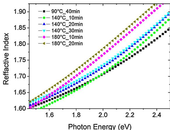
Fig. 3. The refractive indices of solution processed TBADN + NPB:DPAVBi films.
