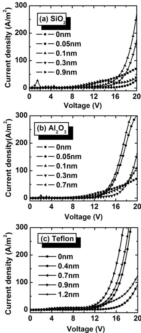
Fig. 2. Current density–voltage characteristics of a hole-only device with (a) SiO<sub>2</sub>, (b) Al<sub>2</sub>O<sub>3</sub>, and (c) Teflon insulating layers of various thicknesses.
