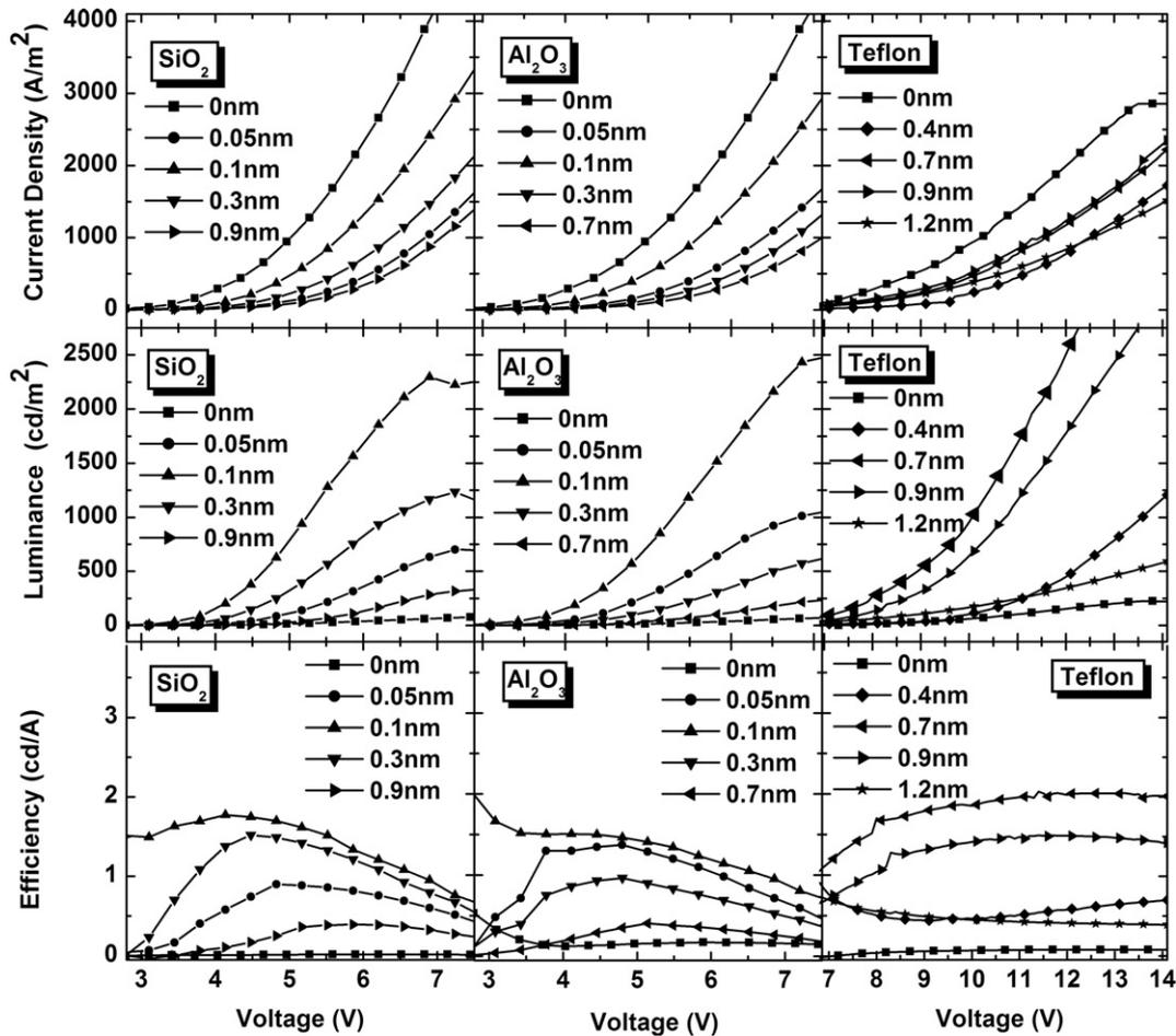
Fig. 1. Current density–voltage, luminance–voltage, and current efficiency–voltage characteristics of single layer OLEDs with  $\text{SiO}_2$ ,  $\text{Al}_2\text{O}_3$ , and Teflon insulating layers of various thicknesses.
