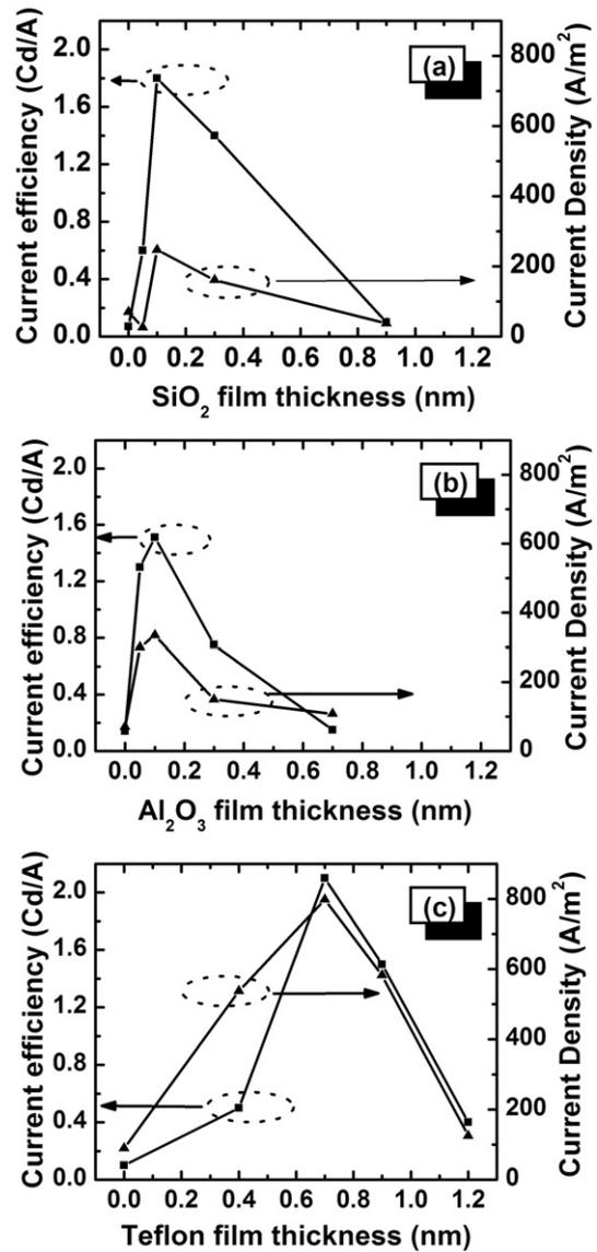
Fig. 3. Hole current density of "hole-only" devices (▲) and C-E of the single-layer OLEDs (■) using different insulating layers (SiO<sub>2</sub>, Al<sub>2</sub>O<sub>3</sub>, and Teflon) with various thicknesses.
