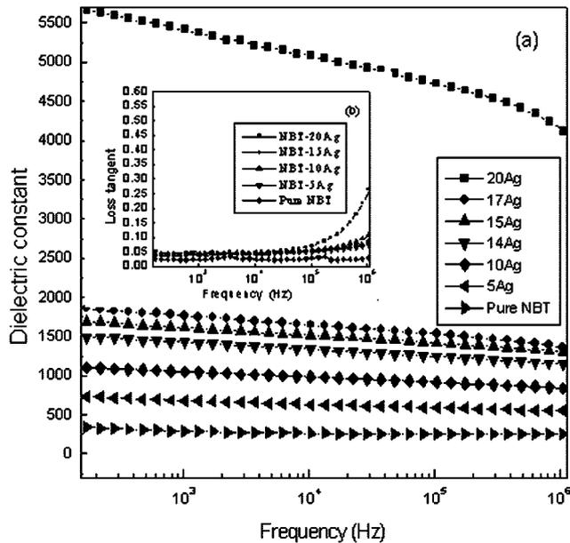
Fig. 3. Frequency dependence of (a) the dielectric constant and (b) loss tangent of the NBT- $x$ Ag composites.
