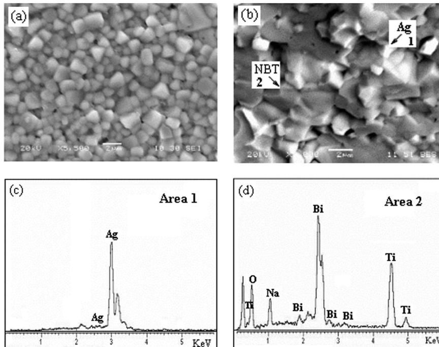
Fig. 2. SEM micrographs of (a) as-fired and (b) fracture surface of the NBT–15Ag sample sintered at 900°C for 2 h. EDX spectra of (c) selected area 1 and (d) area 2 marked in (b).
