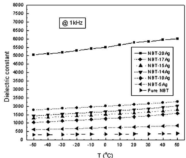
Fig. 5. Variation of the dielectric constant of the NBT- $x$ Ag composites with temperature.
