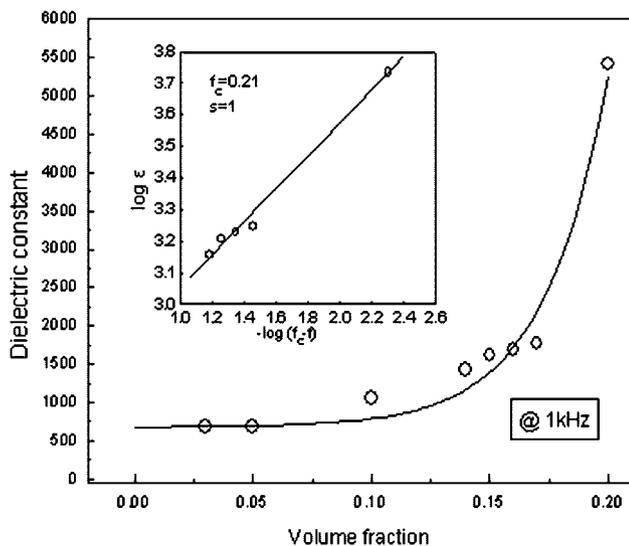
Fig. 4. Dielectric constant of NBT- $x$ Ag composites as a function of volume fraction of silver with logarithmic plot of Eq. (1).
