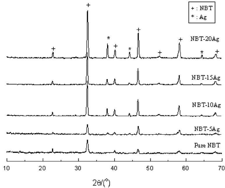
Fig. 1. XRD patterns of different NBT–Ag samples sintered at 900°C for 2 h.
