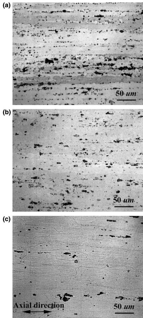
Fig. 3. Typical micrographs of the sectioned Al-Cu-Mg rod treated with (a) TS, (b) TF, and (c) EF.
