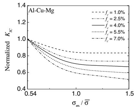
Fig. 9. Calculated dependence of the fracture toughness ( $K_{IC}$ ) on the stress triaxiality level ( $\sigma_m/\bar{\sigma}$ ) for Al–Cu–Mg alloy as a function of the volume fraction of the constituents ( $f_c$ ).
