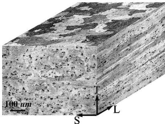
Fig. 2. Triplanar optical micrograph of the Al–Cu–Mg plate and the definition of orientations.
