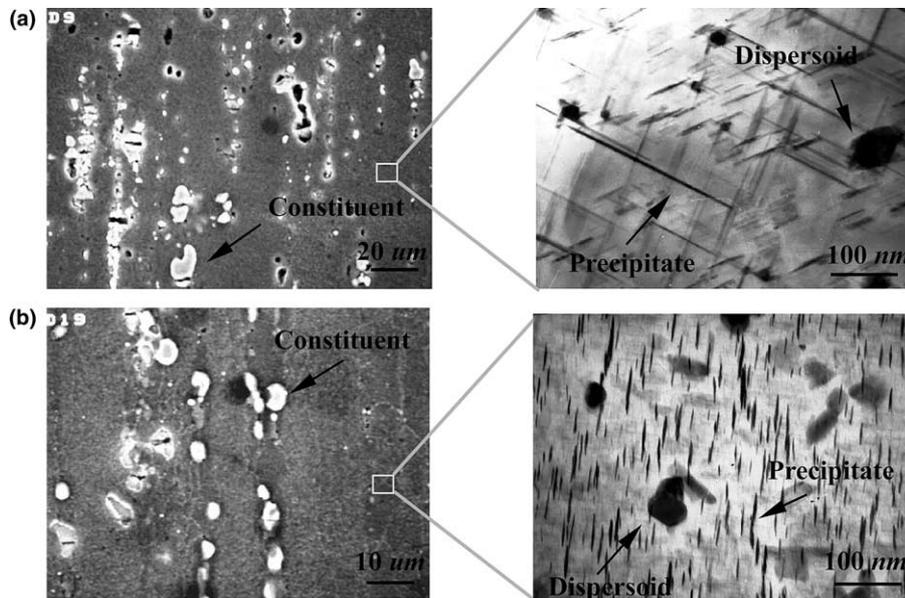
Fig. 1. SEM and TEM images illustrating the three kinds of second phase particles with different sizes and morphologies in the (a) Al–Cu–Mg alloy and (b) Al–Mg–Si alloy.
