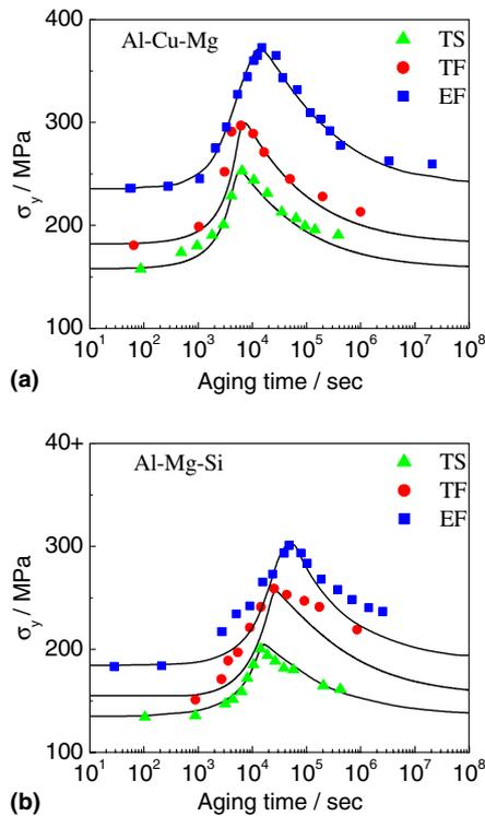
Fig. 5. Variation of yield strength ( $\sigma_y$ ) with aging time for (a) Al–Cu–Mg alloy and (b) Al–Mg–Si alloy. The triangle dots (green), solid dots (red), and square dots (blue) are the experimental results of specimens treated with TS, TF, and EF, respectively. The curves are calculated by using the strengthening model [17]. (For interpretation of the references in colour in this figure legend, the reader is referred to the web version of this article.)
