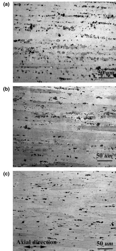
Fig. 4. Typical micrographs of the sectioned Al-Mg-Si rod treated with (a) TS, (b) TF, and (c) EF.
