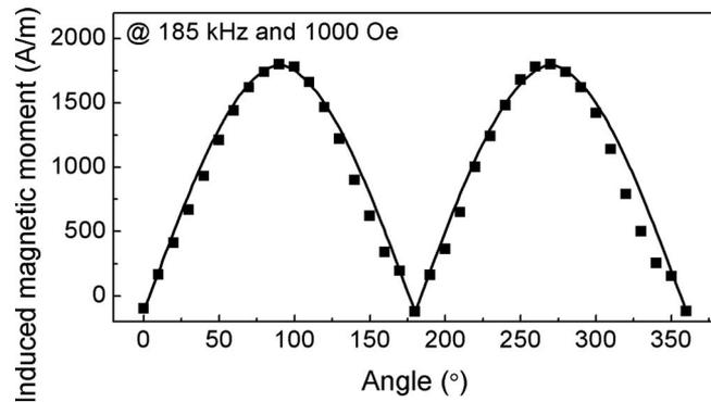
FIG. 4. Dependence of the EIM on the angle  $\theta$  between the polarization and magnetic field. The line is fitted by using Eq. (3).
