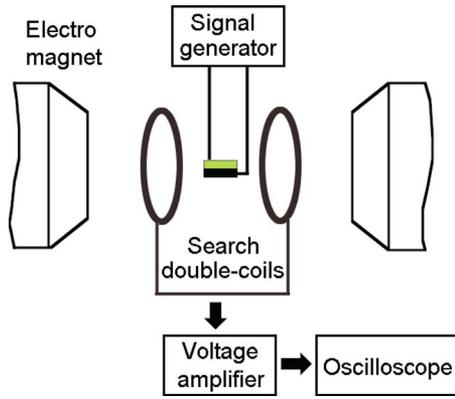
FIG. 1. (Color online) Schematic illustration of the testing setup for EIM measurement.
