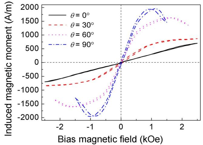
FIG. 3. (Color online) EIM hysteresis loops of the composite in different directions under electric field of 80 V/cm at 185 kHz.
