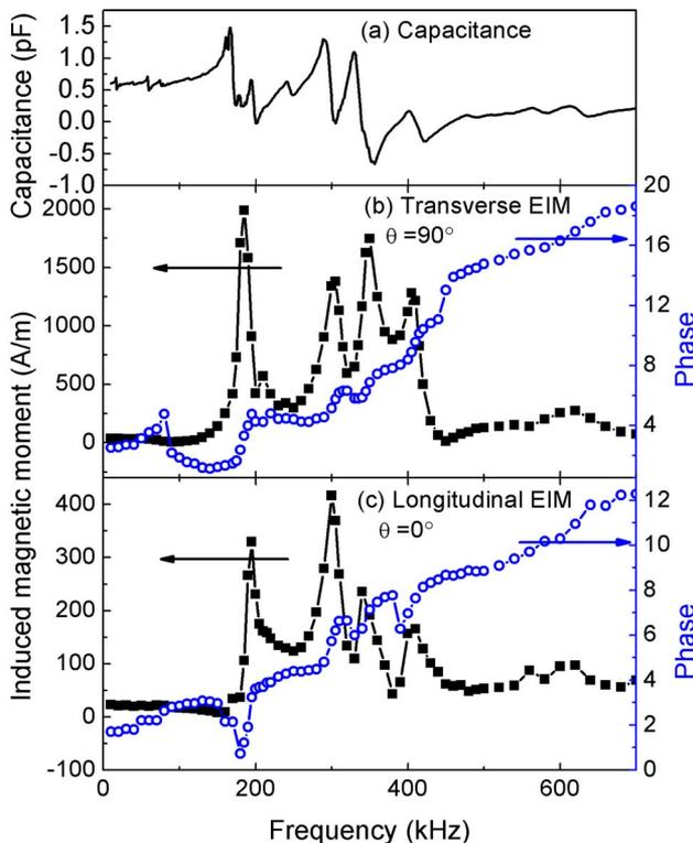
FIG. 2. (Color online) (a) Frequency dependence of composite capacitance. (b) Transverse and (c) longitudinal EIM responses and phasic differences of the laminate composite as functions of frequency under electric field of 83 V/cm and bias magnetic field of 1000 Oe.
