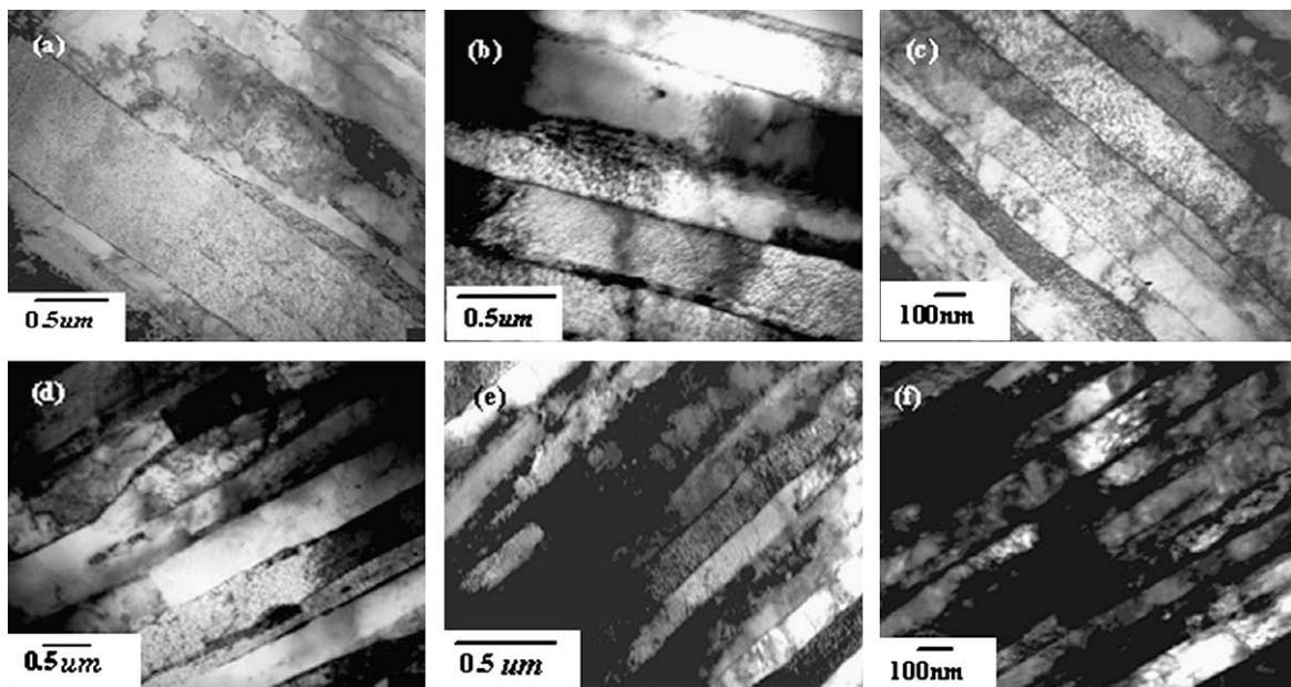
Fig. 1. Transmission electron micrographs of heat-treated lanthanum oxide doped molybdenum alloy wires (a) doped 0.9% La<sub>2</sub>O<sub>3</sub>, 1.5mm diameter, (b) doped 0.9% La<sub>2</sub>O<sub>3</sub>, 0.6mm diameter, (c) doped 0.9% La<sub>2</sub>O<sub>3</sub>, 0.28mm diameter, (d) doped 2.5% La<sub>2</sub>O<sub>3</sub>, 1.5mm diameter, (e) doped 2.5% La<sub>2</sub>O<sub>3</sub>, 0.6mm diameter, (f) doped 2.5% La<sub>2</sub>O<sub>3</sub>, 0.28mm diameter.
