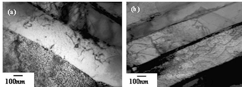
**Fig. 3.** Transmission electron micrographs of dislocations and lanthanum oxide particles in lanthanum oxide doped molybdenum alloy wire (a) doped 0.9%  $\text{La}_2\text{O}_3$ , 0.6mm diameter, (b) doped 2.5%  $\text{La}_2\text{O}_3$ , 0.6mm diameter.
