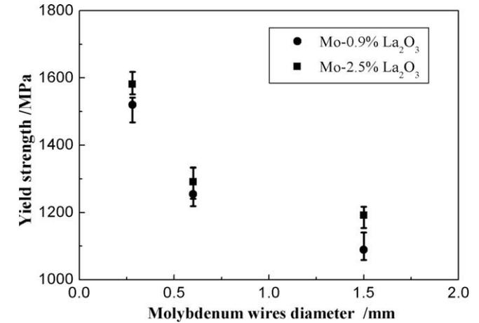
Fig. 2. The yield strength of the molybdenum alloy wires with different mass fractions of lanthanum oxide and different diameter.
