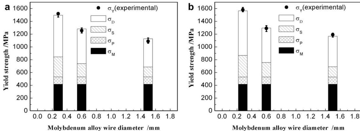
**Fig. 4.** The consist of calculated strength and the comparison of the theoretical strength and experimental strength of the molybdenum alloy wires doped with (a) 0.9wt%  $\text{La}_2\text{O}_3$  and (b) 2.5wt%  $\text{La}_2\text{O}_3$  particles.
