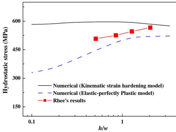
Fig. 3. Dependence of hydrostatic stress on aspect ratio of Cu interconnects (lines), predicted by using elastic-perfectly plastic model and kinematic strain hardening model, respectively. The experimental results from Rhee's [20] are also shown for comparison (dots).
