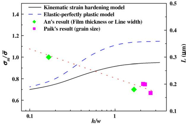
Fig. 4. Dependence of stress triaxiality level on aspect ratio of Cu interconnects (left Y-axis) (lines), predicted by using elastic-perfectly plastic model and kinematic strain hardening model, respectively. Some experimental results [10,26] are presented in this figure to show the dependence of  $L$  on aspect ratio (right Y-axis) (dots).
