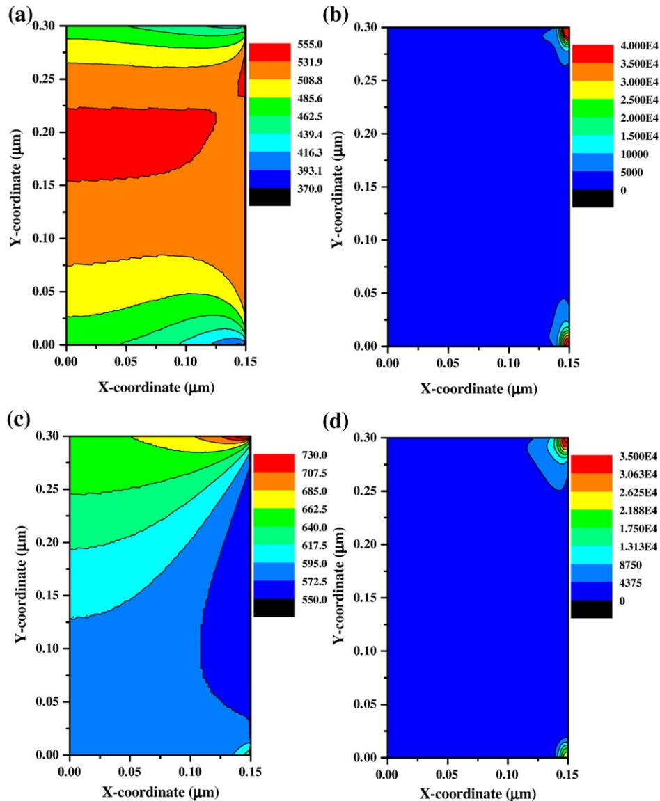
**Fig. 2.** Hydrostatic stress distribution (a and c) and hydrostatic stress gradient contours (b and d) in Cu interconnects with aspect ratio of 1. (a) and (b) are from the elastic-perfectly plastic model while (c) and (d) from kinematic strain hardening model.
