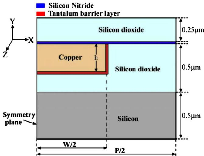
**Fig. 1.** Schematic showing the half of cross section of a periodic unit cell of a passivated Cu interconnects.
