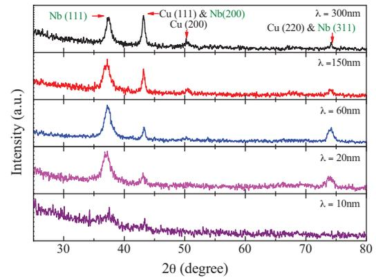
**Fig. 1.** The XRD spectra of Cu/Nb NMFs showing the fcc-Nb with (111) diffraction peak and the fcc-Cu with (111) and (200) diffraction peak.
