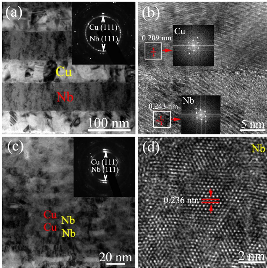
**Fig. 2.** Bright-field cross-sectional TEM micrograph typically showing the modulation structure of the Cu/Nb NMFs with (a)  $\lambda = 150$  nm and (c)  $\lambda = 20$  nm. (b) and (d) are HRTEM images typically showing the crystal structure of Cu/Nb and fcc-Nb layer. Inserts in (a) and (c) are the corresponding selected area diffraction pattern (SADP). Inserts in (b) are the FFT for Cu and Nb of the squared box area, respectively.
