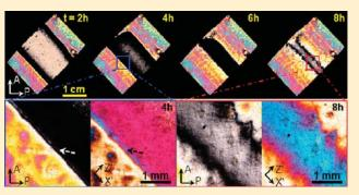
*in situ* the gelation process, an extraordinary molecular reorientation of PBDT at the  $Ca^{2+}$  diffusion flux front is observed for the first time. The mechanism for the molecular reorientation is discussed in terms of complexation and gelation.
