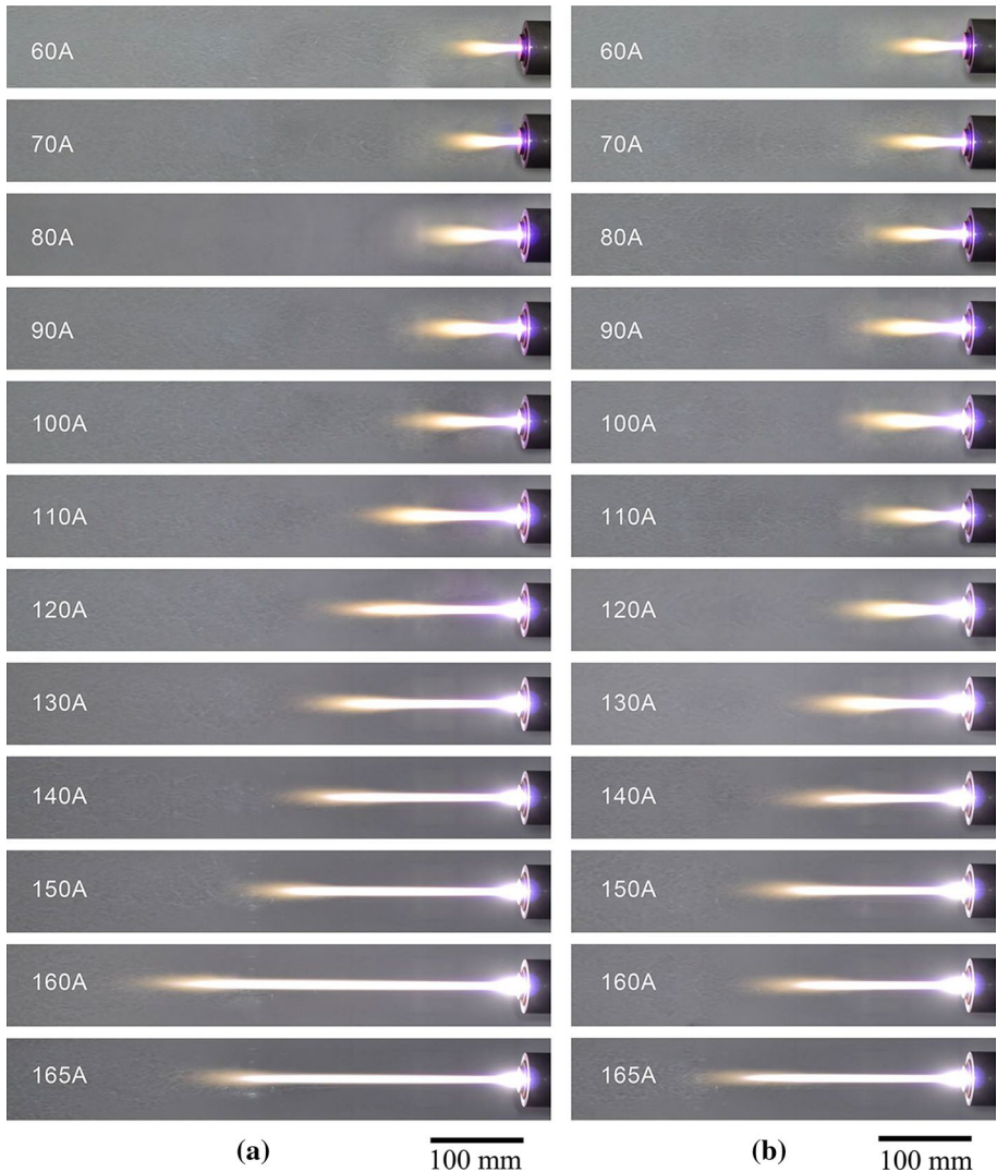
Fig. 3 Laminar plasma jet, showing variation in length for different working current. a Gas flow rate of 14 L min -1 ; b gas flow rate of 15 L min -1
