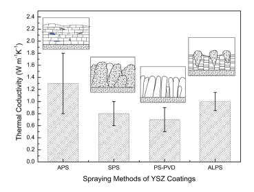
Fig. 4. Thermal conductivities at the room temperature of the YSZ coatings from four plasma spraying technologies.
