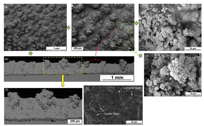
Fig. 3. Top surfaces (a, b, c, d), polished cross sections (e, f) and fracture surface (g) of YSZ coating at the spraying distance of 250 mm.
