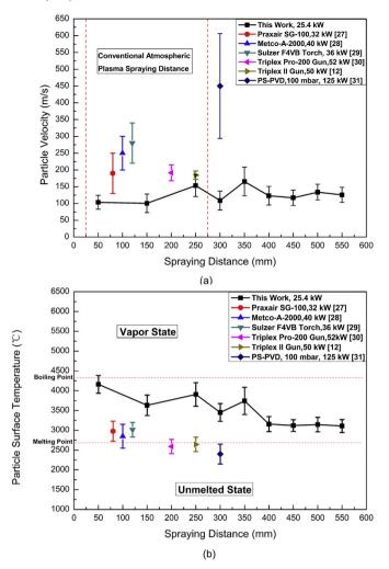
**Fig. 2.** Particle velocity (a) and particle surface temperature (b) in laminar plasma jet at different positions from the nozzle exit and comparison with the results from other plasma spray methods.
