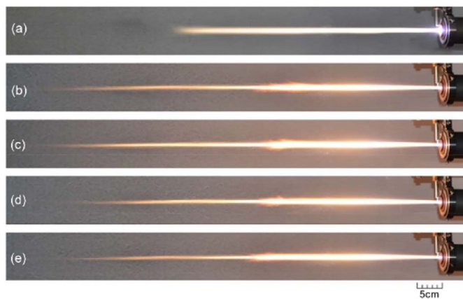
Fig. 4. Photos of laminar plasma jet without particles (a) and with particles heating and acceleration over four consecutive seconds, after 1 s (b); 2 s (c); 3 s (d) and 4 s (e).
