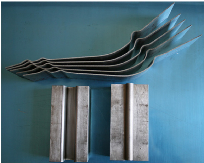
Fig. 7. Experiment results and inserts of draw-bead test device.
