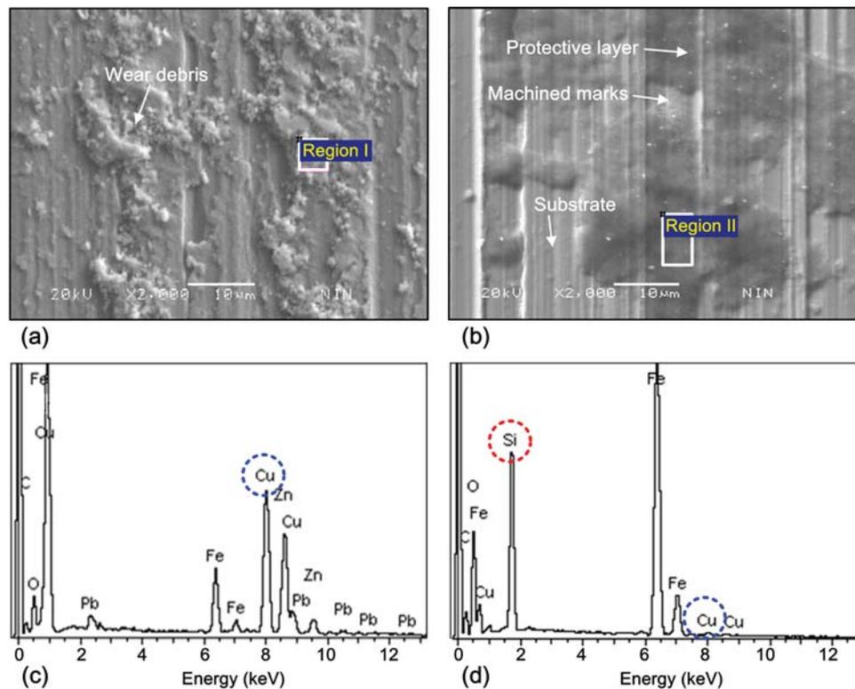
**Fig. 8 Analysis results of the worn surfaces on the disks. (a) and (b): SEM micrographs of the worn surfaces under pure gas film lubrication and NLGF lubrication (nanoparticles concentration:  $58 \text{ g/m}^3$ ), respectively. (c) and (d): EDS spectra of the region I and II, respectively.**
