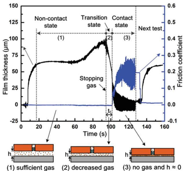
Fig. 3 Variation curves of the film thickness and the friction coefficient during the friction coefficient test (load:  $40 \text{ N}$ ; speed:  $100 \text{ rpm}$ ; nanoparticles concentration:  $32 \text{ g/m}^3$ )
