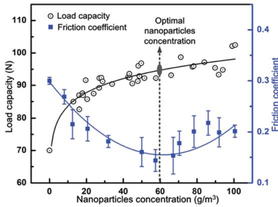
Fig. 5 Load capacity and friction coefficient with different nanoparticle concentrations
