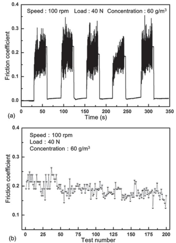
Fig. 7 Variation of the friction coefficient in the start-stop cyclic test
