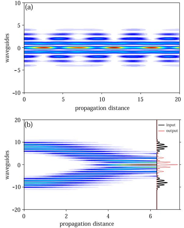
**Figure 3.** (a) Propagation of a Gaussian beam in a  $\Lambda$ -type modulated waveguide array with the zero waveguide excited by the beam peak. A Fermi–Pasta–Ulam recurrence-like oscillation happens during propagation. (b) Two Gaussian beams launched from positive and negative waveguide sides coalesce during propagation. The curves in the right panel depict the corresponding beam intensities at the input and output places, respectively.
