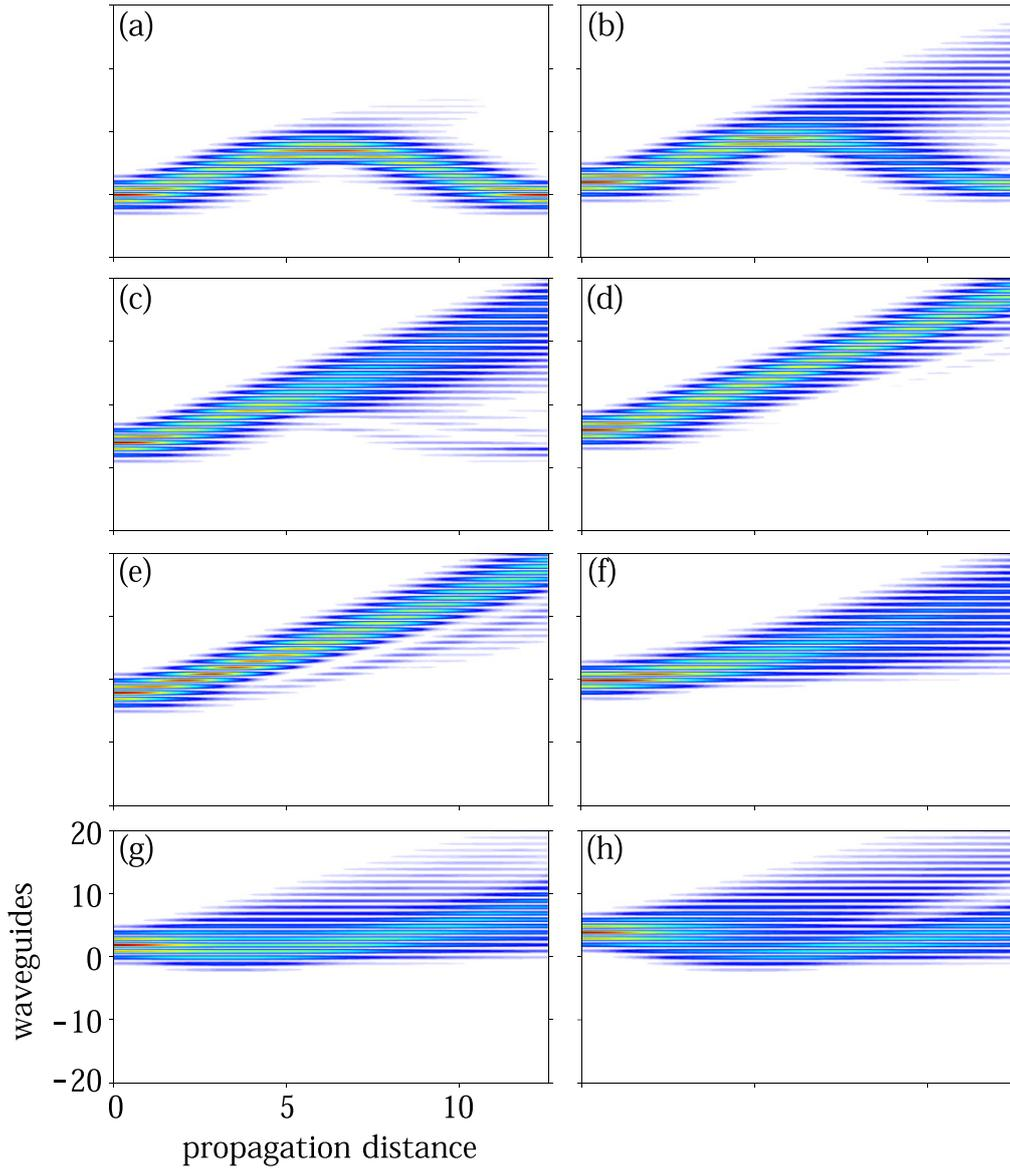
**Figure 1.** Propagation of a Gaussian light beam in a periodic waveguide array with  $\alpha = 0.5$  for  $m \leq 0$  and  $\alpha = 0$  for  $m > 0$ . (a)–(h) Peaks of the incident beams are located at waveguides  $-10, -8, -6, -4, -2, 0, 2,$  and  $4$ , respectively.
