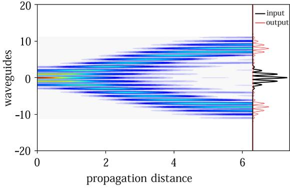
**Figure 2.** A Gaussian beam splits during propagation in a V-type modulated waveguide array. The zero waveguide is excited by the beam peak. The curves in the right panel are the corresponding beam intensities at the input and output places, respectively.
