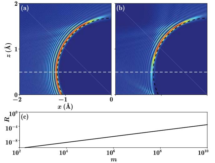
Fig. 1. (a) Propagation of a half-Bessel beam that accelerates along a circular trajectory. The black dashed curve indicates the theoretical accelerating trajectory, and the white dashed line the axis of symmetry of the trajectory. (b) Self-healing of the beam when the main lobe is removed. (c) Dependence of  $R$  on the order  $m$  of the half-Bessel beam.
