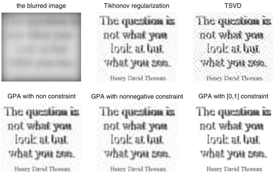
Fig. 1 Comparison of TSVD, Tikhonov regularization and Gradient projection algorithm for image deblurring
