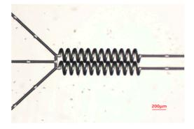
Figure 3. Small spacing structure of a multiple channel mixer.
