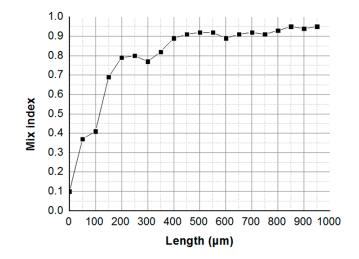
**Figure 6.** Experimental mixing performance of the helical micromixer: mixing index  $\sigma$  graphics of Figure 5a.
