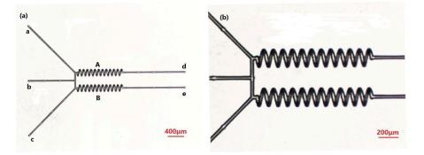
**Figure 2.** (**a**) Morphology of a multiple channel mixer, observed via optical microscope; and (**b**) detail of mixer with enlarged scale.
