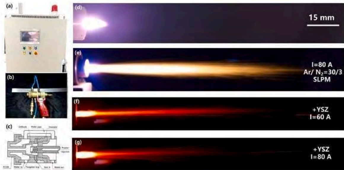
Fig. 16. (a) Power supply unit of the AMPS system; (b) plasma torch and (c) its internal structure [111]; (d, e) experimental plasma jets produced in an atmospheric environment; (f, g) plasma jet with YSZ particles at different input current.
