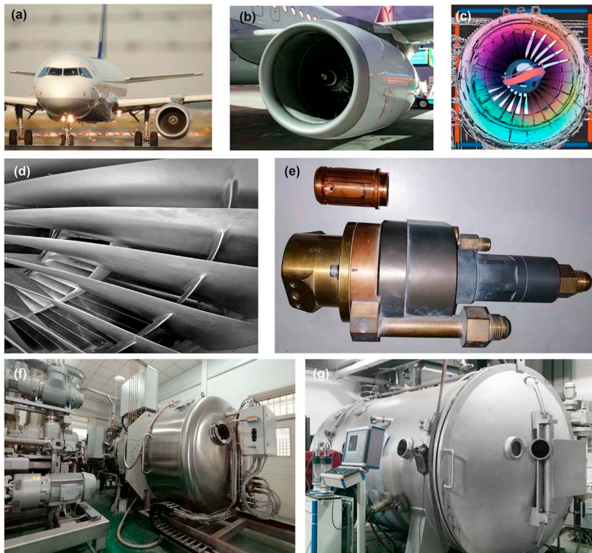
Fig. 1. Applications of thermal barrier coatings in (a), (b), (c), (d); the used plasma torch under the reduced pressure condition (e); the low-pressure plasma spray (LPPS) system at BUAA (f); the low-pressure plasma spray system in XJTU (g) (Copyright © Pixabay Licence).
