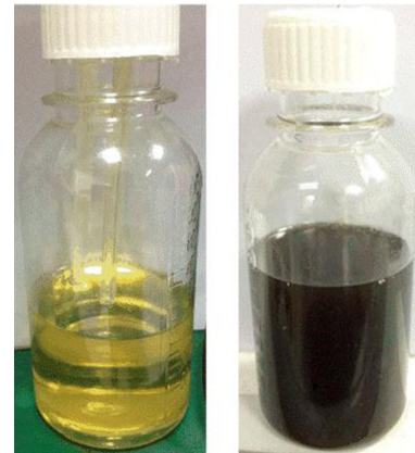
Fig. 10. Oil samples of the new oil (left) and the used oil (right).
