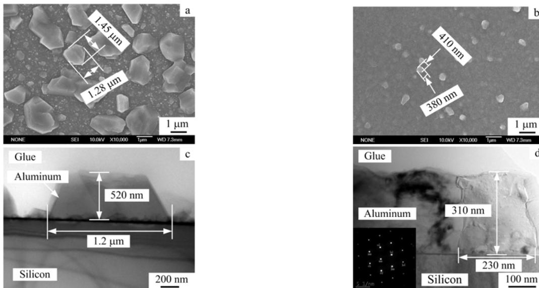
Fig.2 Surface morphologies of ECR-Al films with different substrate biases: (a) +40 V, (b) +20 V; and cross-sectional HRTEM pictures: (c) +40 V, (d) +20 V.
