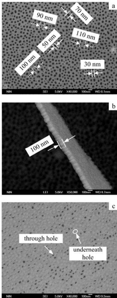
Fig.3 AAF with nano holes. (a) top view, (b) cross-sectional view, (c) backside view
