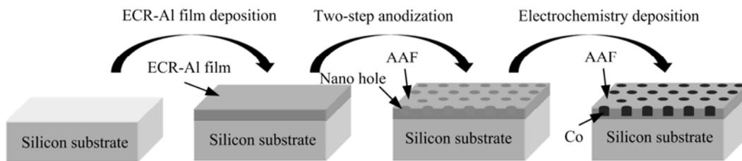
Fig.1 Schematic of the experimental procedures
