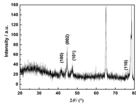
Fig.5 XRD patterns of Co nanodots embedded in AAF
