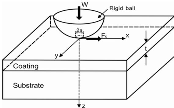
Fig.1 Contact model of ball on layered surface
