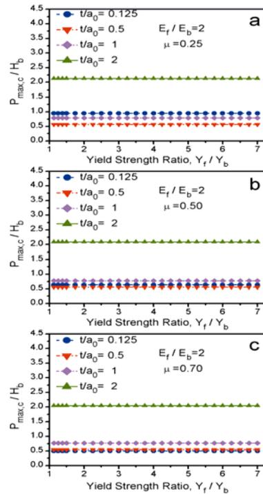
Fig.4 Critical maximum contact pressure for yielding at the interface, (a)  $\mu=0.25$ ; (b)  $\mu=0.50$ ; (c)  $\mu=0.70$
