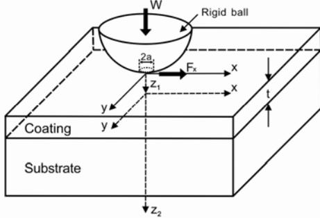
Fig.1 Contact model of a rigid ball on a layered substrate
