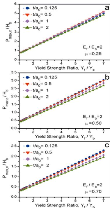
Fig.6 Critical maximum contact pressure for yielding at the surface, (a)  $\mu=0.25$ ; (b)  $\mu=0.50$ ; (c)  $\mu=0.70$
