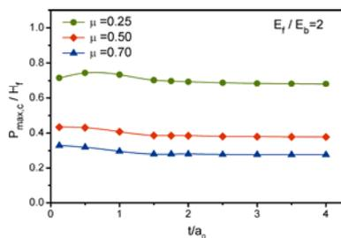
Fig.7 Relationship between the normalized critical maximum contact pressure for yielding at the surface  $P_{max,c}/H_f$  and  $t/a_0$
