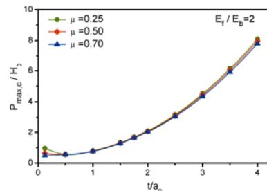
Fig.5 Relationship between the normalized critical maximum contact pressure for the yield at the interface  $P_{max,c}/H_b$  and  $t/a_0$
