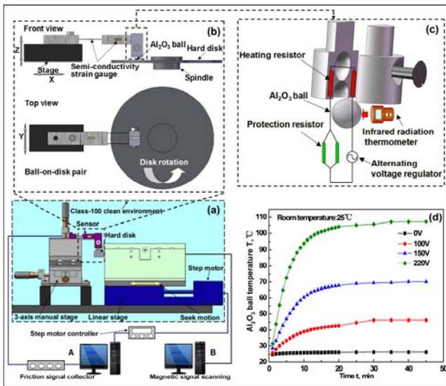
Fig.1 Schematic sketch of ball-on-disk tribo-test apparatus: (a) ball-on-disk loading system; (b) magnetic disk scanning system; (c) heat source system; (d)  $\text{Al}_2\text{O}_3$  ball temperature versus time at different voltages
