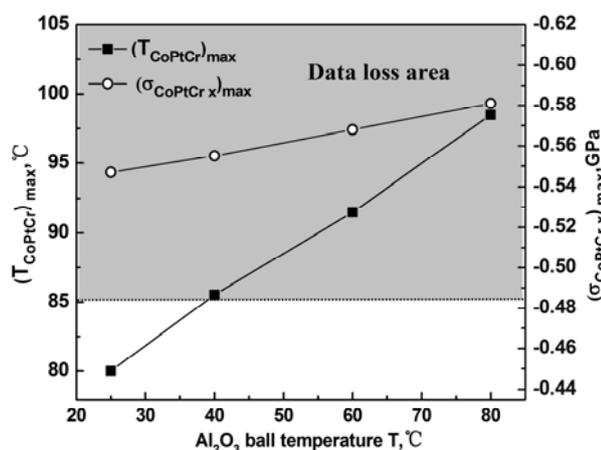
Fig.6 Al<sub>2</sub>O<sub>3</sub> ball temperature versus maximum temperature and stress at different temperatures in disk under heat source sliding contact ( $V = 17.34\text{ m/s}$ ,  $W = 0.025\text{ mN}$ )
