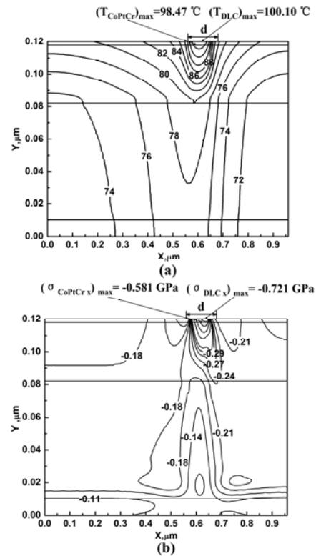
Fig.5 (a) contours of temperature and (b) contours of  $\sigma_x$  in the semi-infinite medium of the disk under heat source sliding contact ( $V= 17.34$  m/s,  $W= 0.025$  mN,  $T= 80$  °C)
