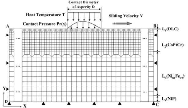
Fig.4 Illustration of finite element model
