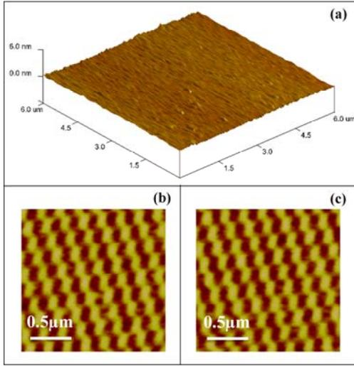
Fig.3 Typical AFM and MFM images of the disk in the contact area after tribo-test ( $V= 17.34$  m/s,  $W= 0.025$  mN,  $T= 80$  °C): (a) 3D AFM image of the disk surface in the contact area; (b) MFM image in the contact area; (c) MFM image outside the contact area
