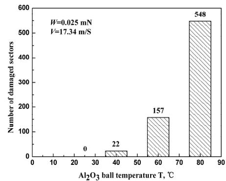
Fig.2 The number of damaged sectors induced by tribo-test at different  $\text{Al}_2\text{O}_3$  ball temperatures
