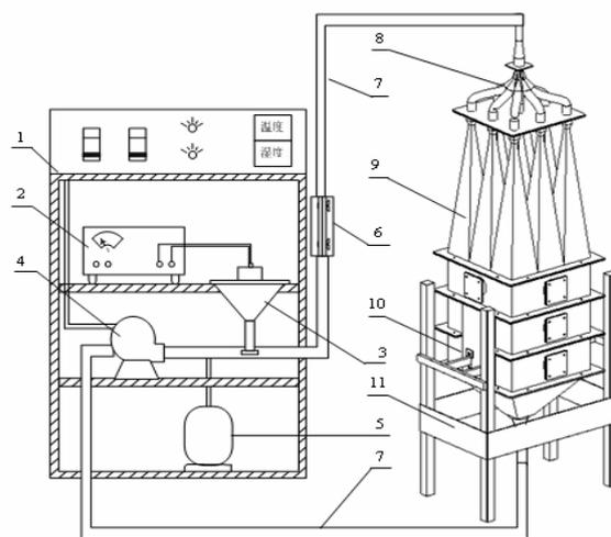
Fig.3 Schematic diagram of the sand dust environment simulator(1-control casing; 2-direct current source; 3- sand supply device; 4-air blower; 5-humidity chamber; 6-secondary filter; 7-blast tube; 8-sand distributor; 9-multi-Venturi diffuser; 10-environment simulator; 11-support frame)
