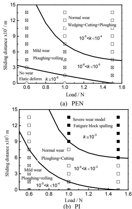
Fig.5 Wear map of polymers in sand dust environment  $k$  - wear rate, mm<sup>3</sup>/N.m
