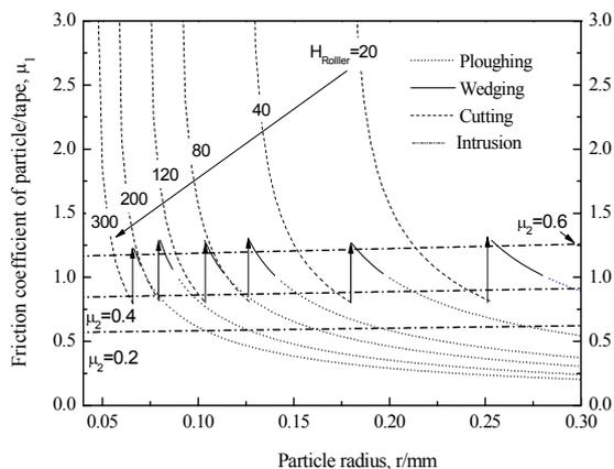
Fig.11 Intrusion conditions corresponding with abrasive wear models of different  $H_{\text{tape}}$ . ( $w = 1$  N ;  $f = 0.2$ )
