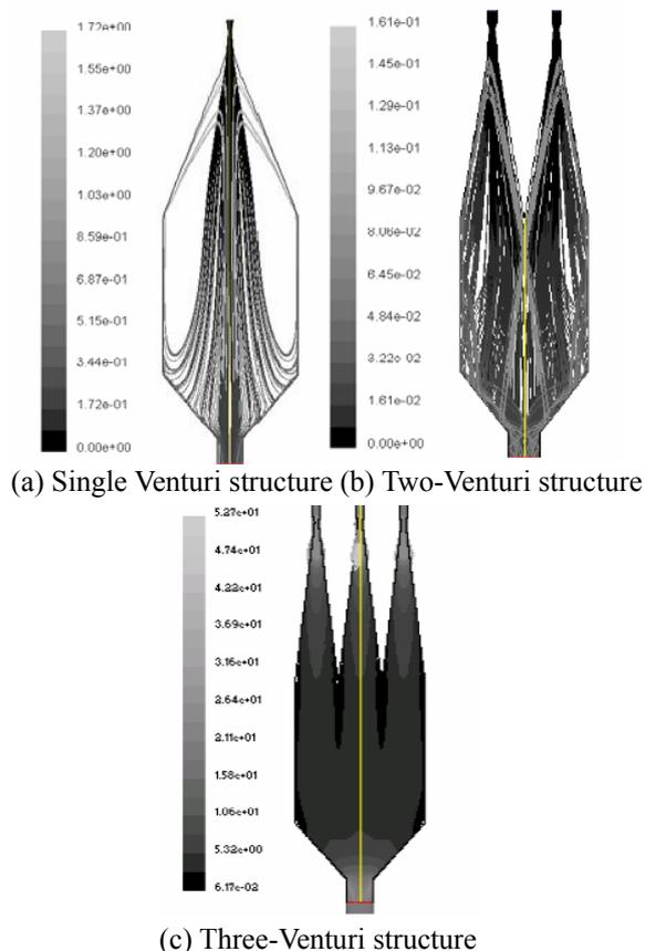
Fig.2 Simulation results of particle tracks in three Venturi structure
