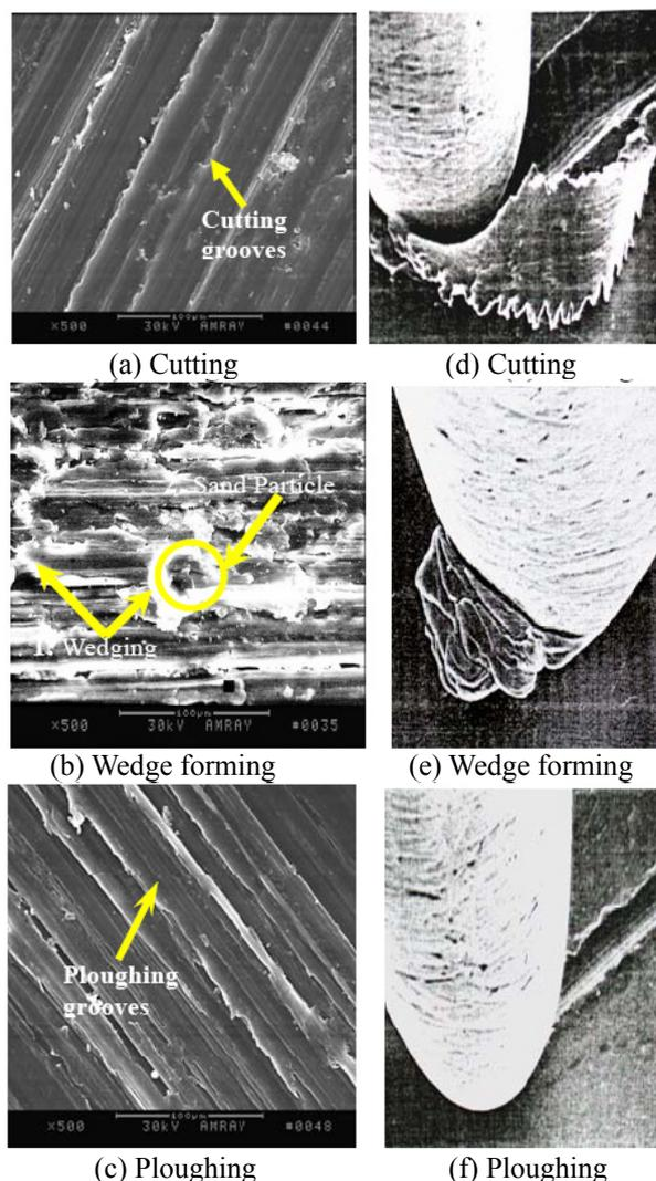
Fig.6 Typical abrasive wear mechanisms of: (a)-(c) polyimide tape; (d)-(f) metal<sup>2)</sup>
