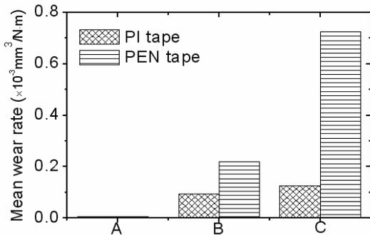
Fig.7 Mean wear rates of PEN and PI tape in clean air environment and in sand storm environments. A-Clean air environment, B-Sand storm environment, C-Severe sand storm environment<sup>1)</sup>
