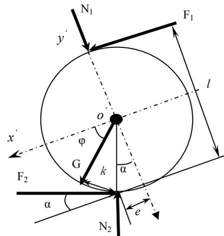
(b) Force diagram of particle in intrusion
