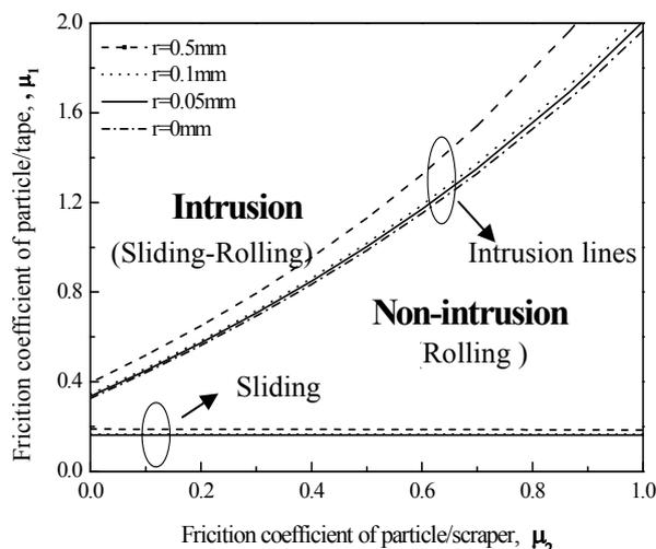
Fig.9 Intrusion pattern map of sphere particle into a contact interface
