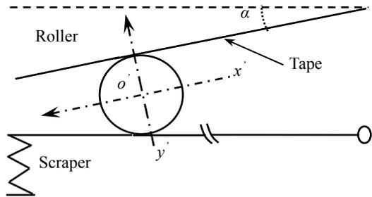
(a) Simplified invasion model of particle into roller-scraper tribosystem
