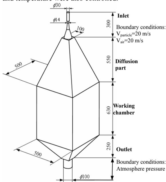
Fig.1 Simulation model with single Venturi structure
