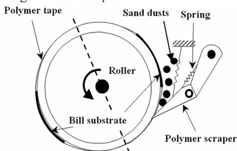
Fig.4 Schematic diagram of ATM roller-scraper tribosystem<sup>1)</sup>
