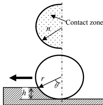
Fig.10 Contact model between hard sphere particle and polymer tape<sup>2)</sup>
