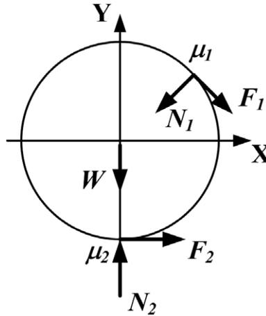
Figure 5. Force distribution at ball surface  $56 \times 69$  mm ( $300 \times 300$  dpi).
