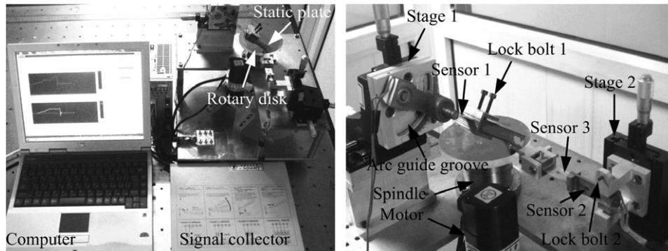
Figure 2. The tribotester of ball intrusion into sliding contact space  $165 \times 60$  mm ( $300 \times 300$  dpi).
