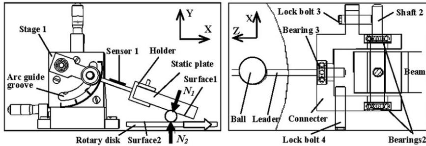
(b) Structure of the static plate and its holder (c) Connect method of ball, connector and beam
