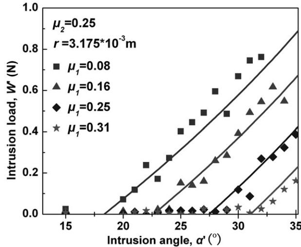
Figure 7. Experimental and calculating results of intrusion load and intrusion angle under different friction coefficients of  $\mu_1$ , ( $\mu_2 = 0.25$ )  $151 \times 123$  mm ( $300 \times 300$  dpi).
