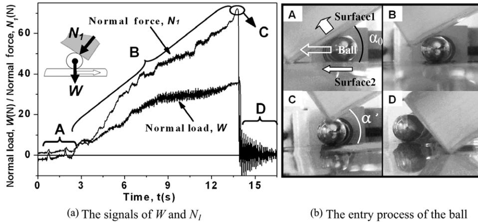
Figure 3. Normal load putting on the centre of the ball and normal force between the ball and surface 2,  $164 \times 75$  mm ( $300 \times 300$  dpi).
