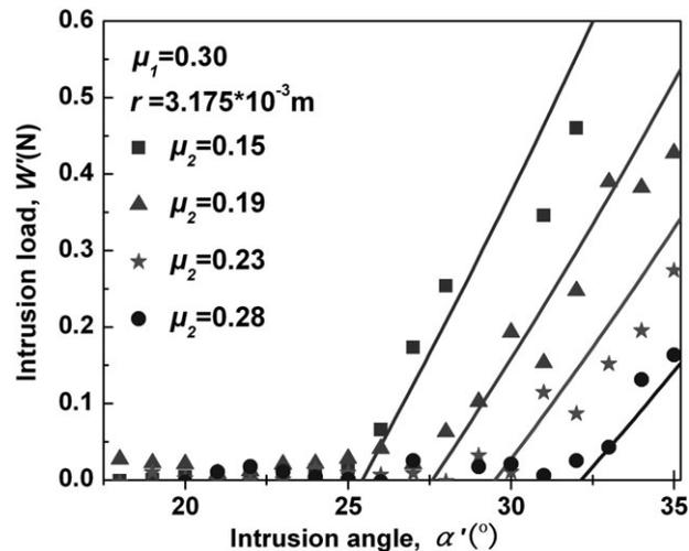
Figure 6. Experimental and calculating results of intrusion load and intrusion angle under different friction coefficients of  $\mu_2$ , ( $\mu_1 = 0.3$ )  $150 \times 118$  mm ( $300 \times 300$  dpi).
