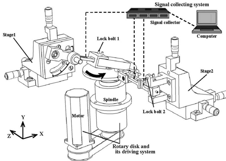
(a) The integrated schematic drawing of the tribotester
