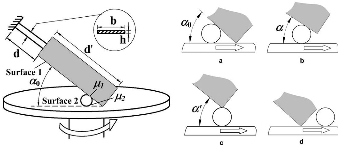
Figure 4. The sliding contact space model for simulating a ball intrusion into a space  $161 \times 71$  mm ( $300 \times 300$  dpi).
